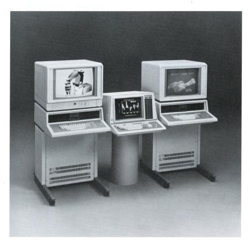
drive is required. The Winchester disk can store up to 10M bytes of data, and up to 4 drives can be connected to the terminal. Each 8-inch flexible disk provides up to 494K bytes of file storage.
