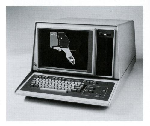
The 4112 offers a bright, flicker-free 381mm (15-inch) raster scan display with a viewable resolution of  $640 \times 480$  points, augmented by  $4096 \times 4096$  point addressability and by zoom and pan.
