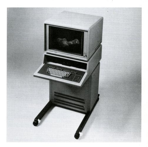
4096Y addressable points (4096X by 3120Y displayable points) provide resolution high enough for the most complex engineering and scientific graphics. The 4114 offers enhanced text display with as many as 16 hardware-generated sizes of stroke upper-and-lower case ASCII characters. A large number of dotdash line styles and markers, plus rubberbanding capability, simplify graphics development. Thumbwheel-controlled symbols enable easy placement and revision of display elements.
