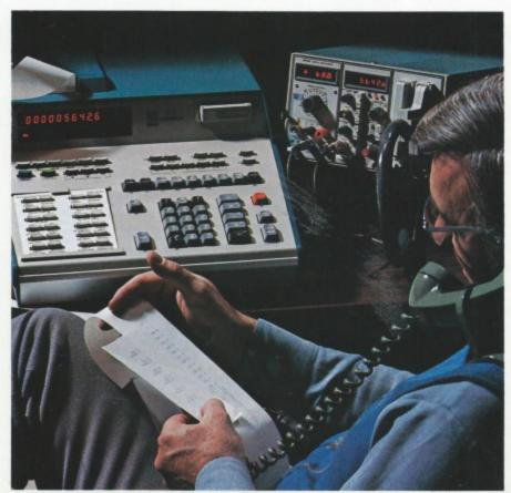
instrumentation interface with built-in power supply, a digital translator and any of our compact digital multimeters and counters. Each mainframe holds two plug-ins, and the calculator can control up to 20 plug-ins simultaneously.
