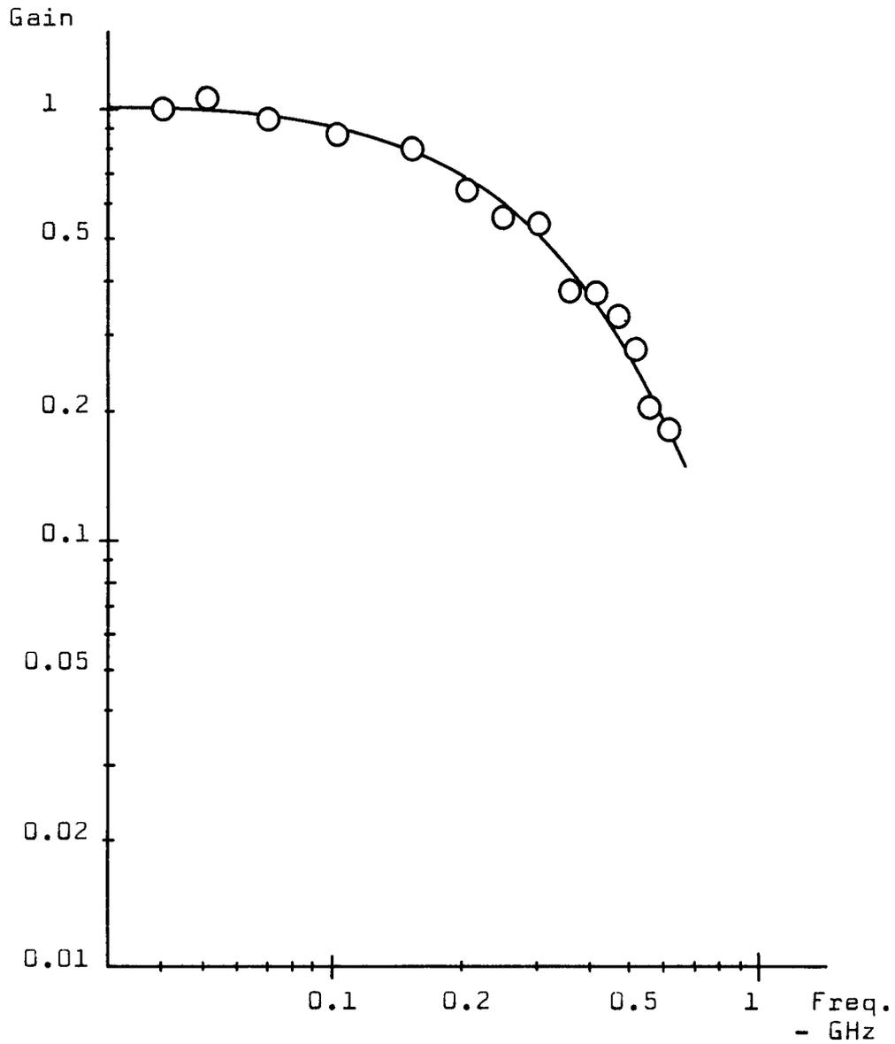
Fig. 14 shows normalized incremental gain of the two inputs compared to that of the differential pair alone. The ideal here would be to have a horizontal line of constant incremental gain over the range.
