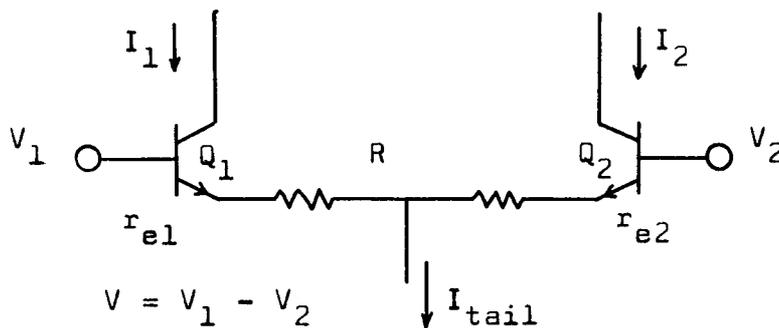
Fig. 8b. Emitter impedance in a differential pair vs. signal.
