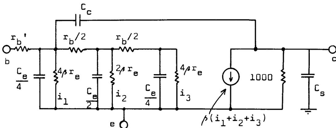
The 1000 ohm resistor was picked arbitrarily, because Ecap requires a resistor on the current source, and all resistors that connect to any one node should be within a range of 1:1000 of each other. This should not make much difference on the bandwidth, since each collector drives a load that is significantly less than 1000 ohms.
