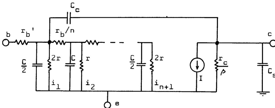
The collector-base capacitance can still be fed back to the bulk resistance of the inactive base region with reasonable accuracy, since very little of it is actually under the active base.
