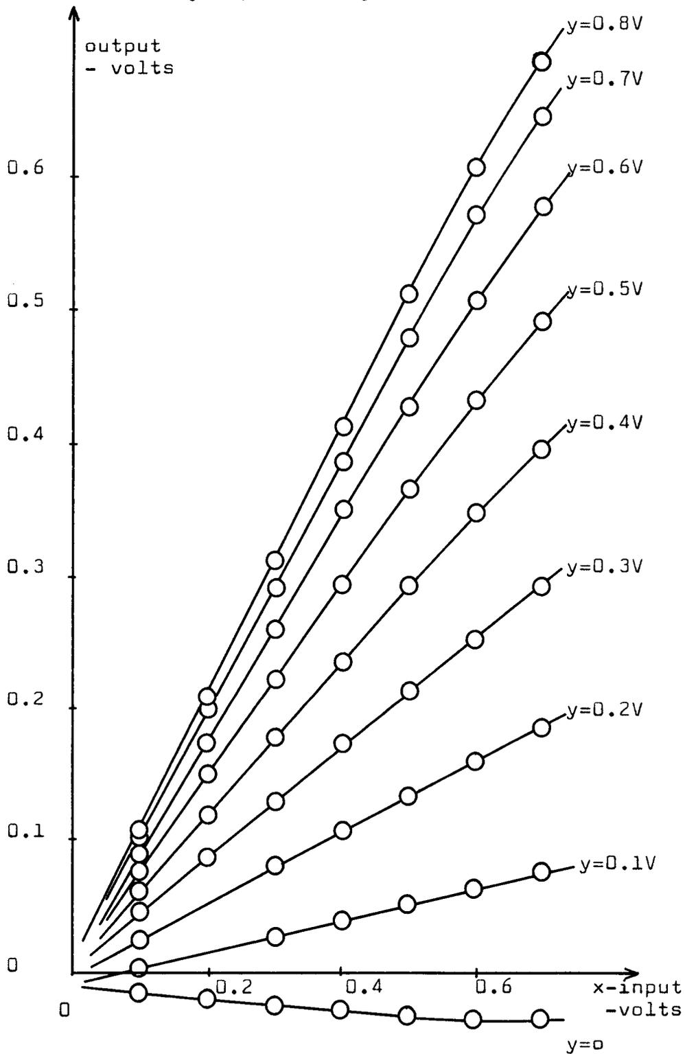
Fig. 13. Measured output in Table 1, shown as output voltage vs. y-input voltage, with x-input voltage as parameter.
