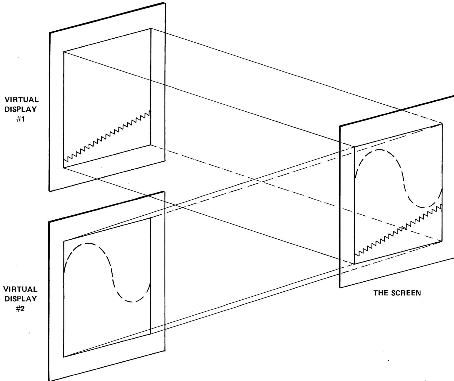
Fig. 3.5. Common Screen Window with several Virtual Displays.
