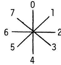
Each incremental plot character will move the beam one raster unit in the given direction.
