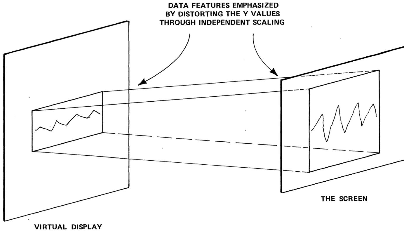
Fig. 3.3. Independent X, Y Window Scaling.
