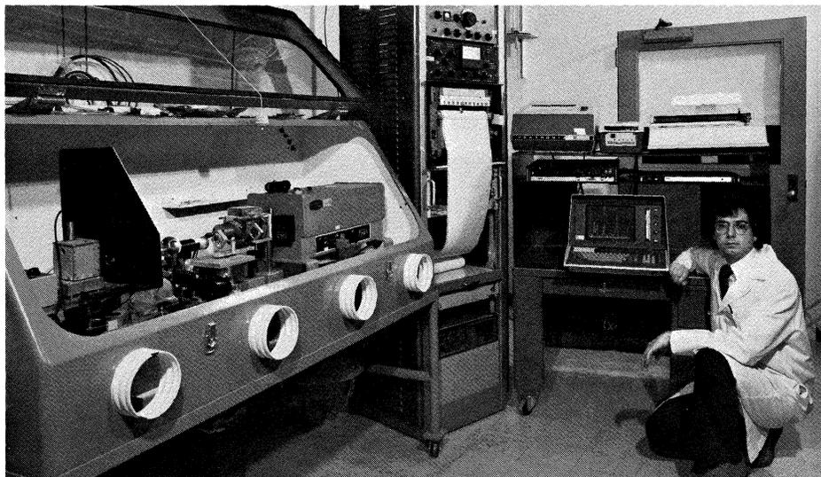
Fig. 2. Microscope spectrophotometer and Tektronix 4051 system.
