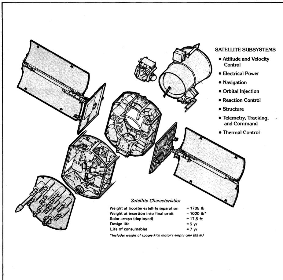
Fig. 2. There are over 33,000 parts in each satellite. Three redundant clocks provide sufficient backup to cover system failures.
