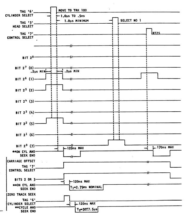
\*\* ON CYL AND SEEK END SIGNALS ARE IDENTICAL UNLESS SEEK ERROR OCCURS. SEEK ERROR INITIATES A CONSTANT SEEK END.
