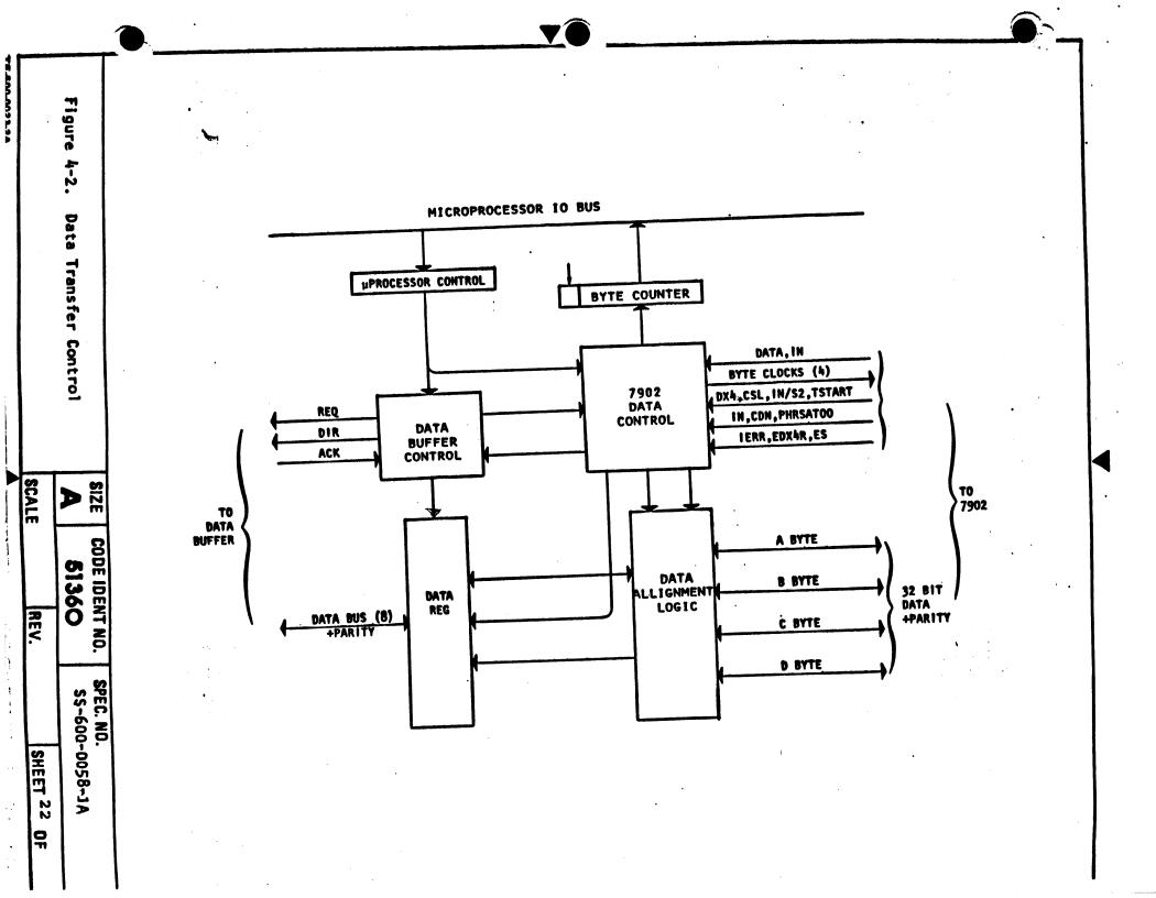
Parity generation and checking will be provided on the data transmitted between the IFX and DATA BUFFER. Any parity error will set a latch which may be monitored by the processor (see 4.2) and will be reported to the IOP as a transmission data error (see 4.7).
