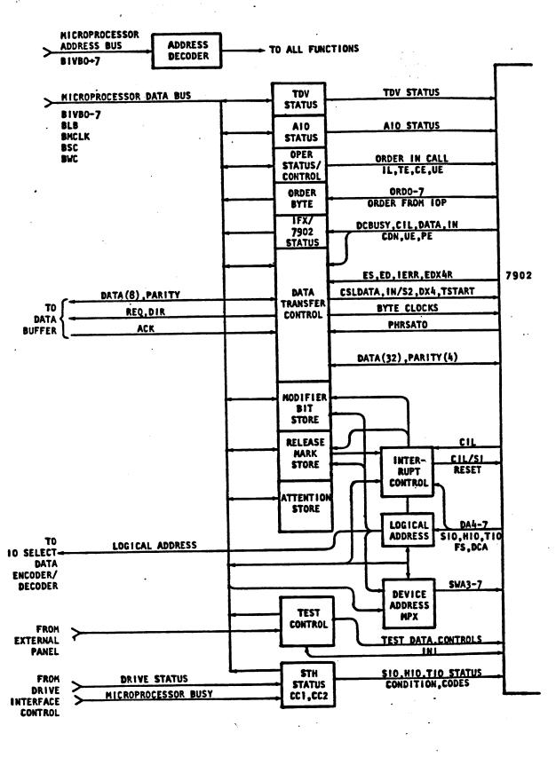
Figure 4-1. IFX/7902 Block Diagram
