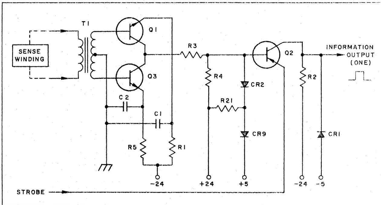
Figure 4-9. Read Amplifier, Simplified Schematic Diagram
