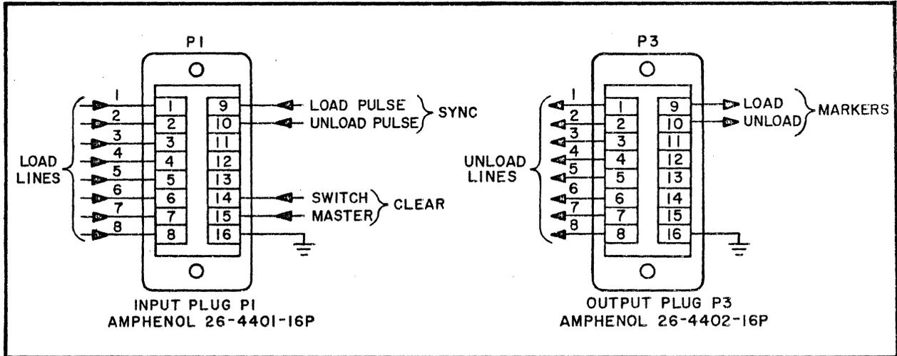
Figure 2-1. Input and Output Connector Wiring For 144-BA-4A, 144-BA-8A, 144-BQ-4A, and 144-BQ-8A Buffers.
