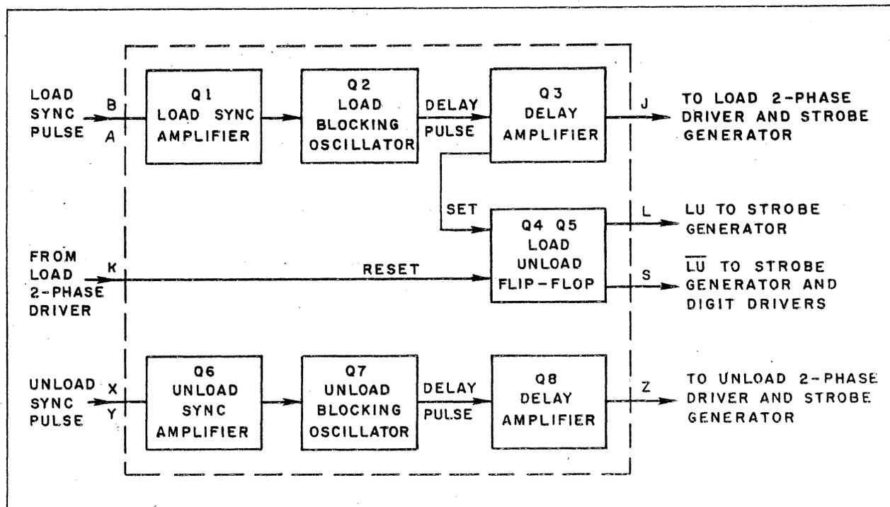
Figure 4-3. Input Sync Amplifier, Block Diagram
