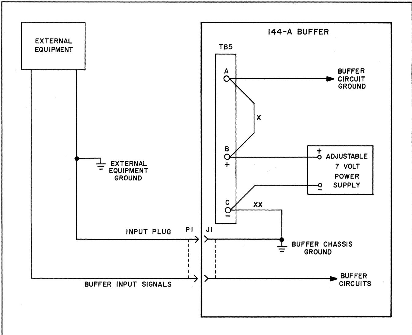
Figure 4-12. Level Shifting By Means of the Circuit Ground
