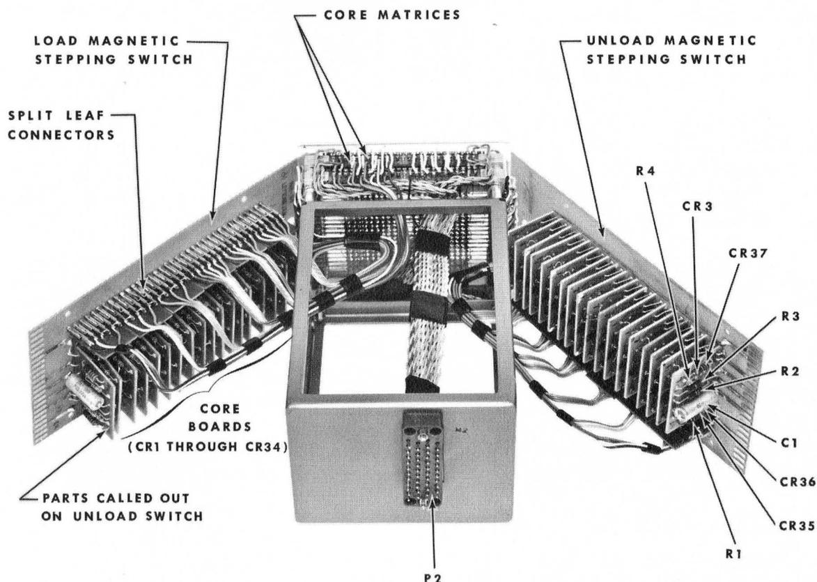
Figure 5-5. Storage System and Magnetic Stepping Switches For 144-BQ-8A Buffer, Parts Identification
