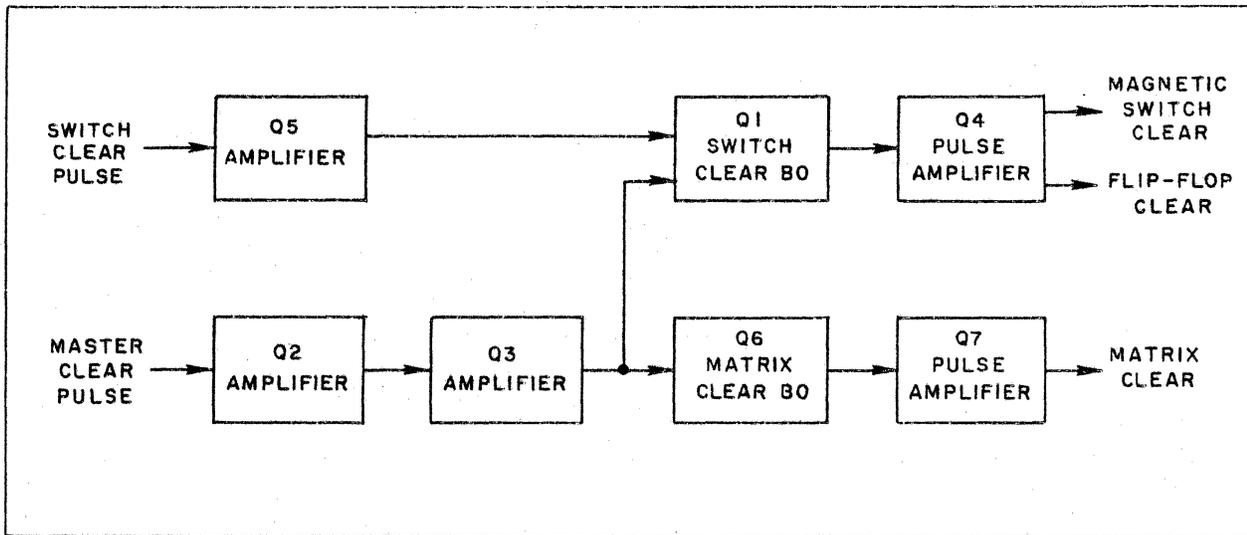
Figure 4-11. Electronic Clear Circuits, Block Diagram
