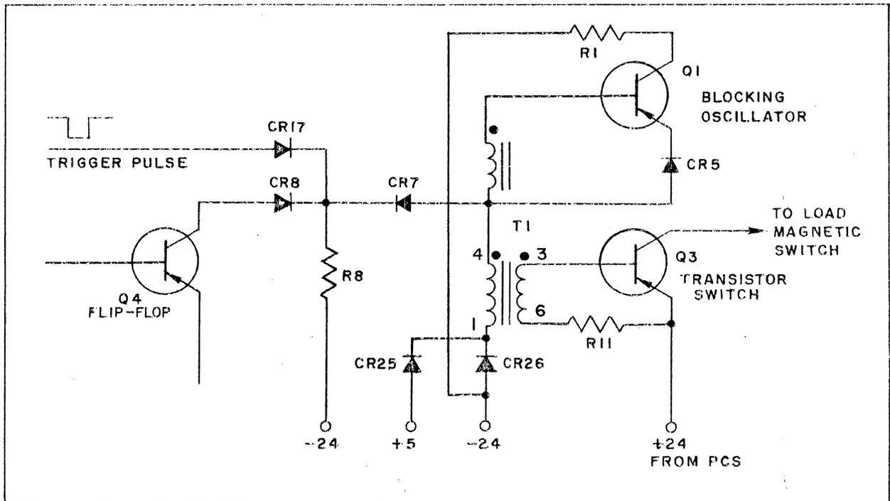
Figure 4-5. AND Gate and Blocking Oscillator, Simplified Schematic Diagram
