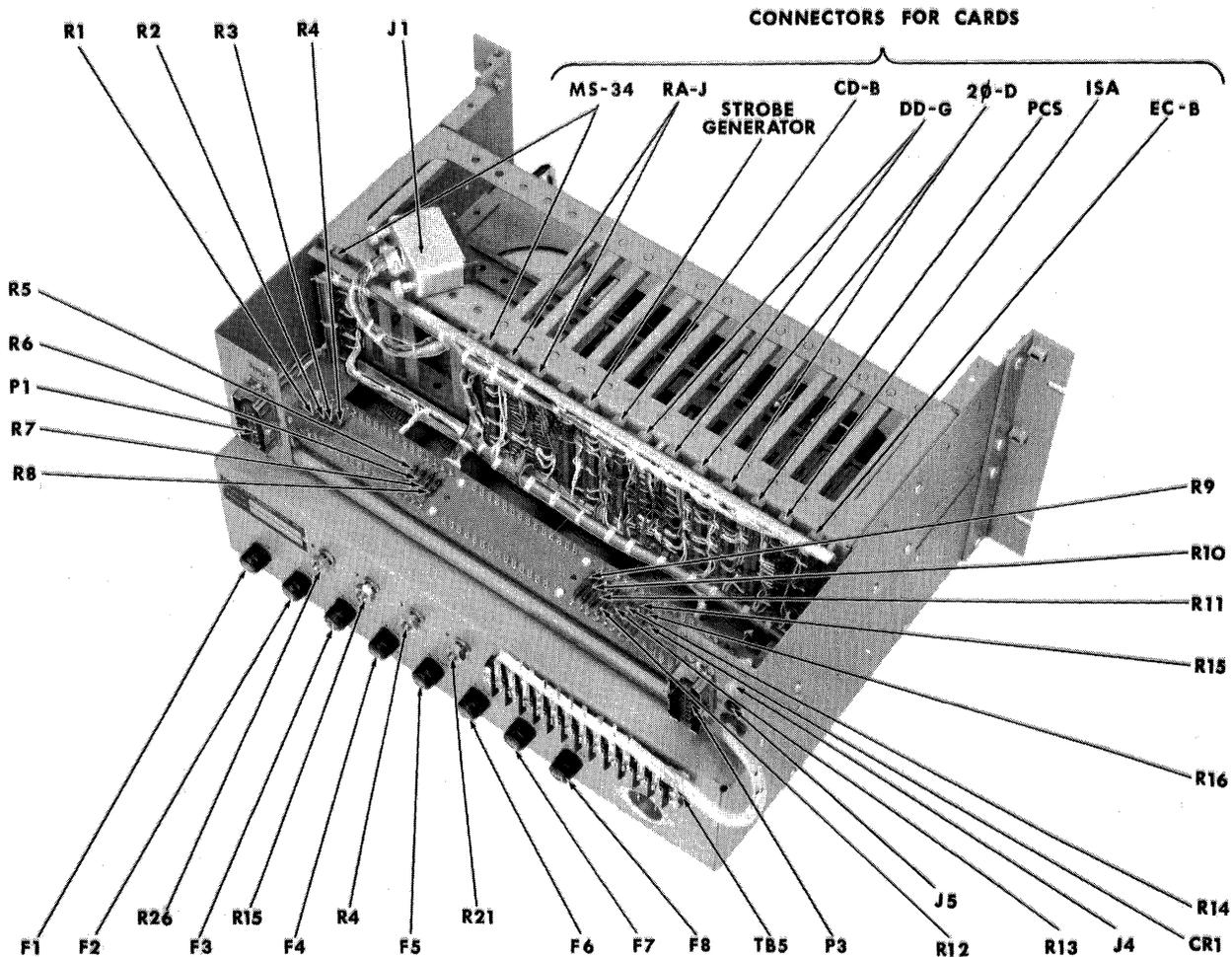
Figure 5-7. Buffer Parts Identification, Storage System, Magnetic Stepping Switches and Printed Circuit Cards Removed
