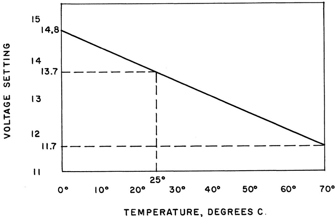
Figure 5-3. Calibration Chart For -14 Volt Output
