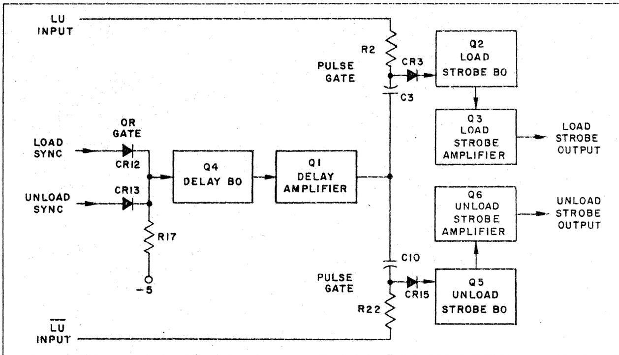
Figure 4-10. Strobe Generator, Functional Block Diagram
