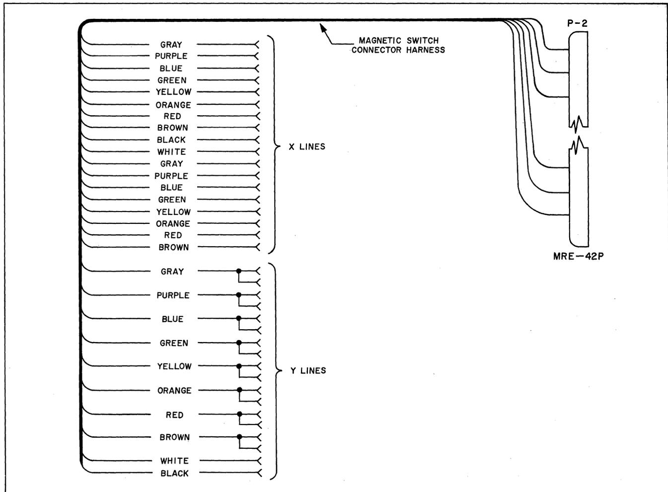
Figure 5-6. Matrix Wiring From Plug P-2 to Magnetic Switch Connectors
