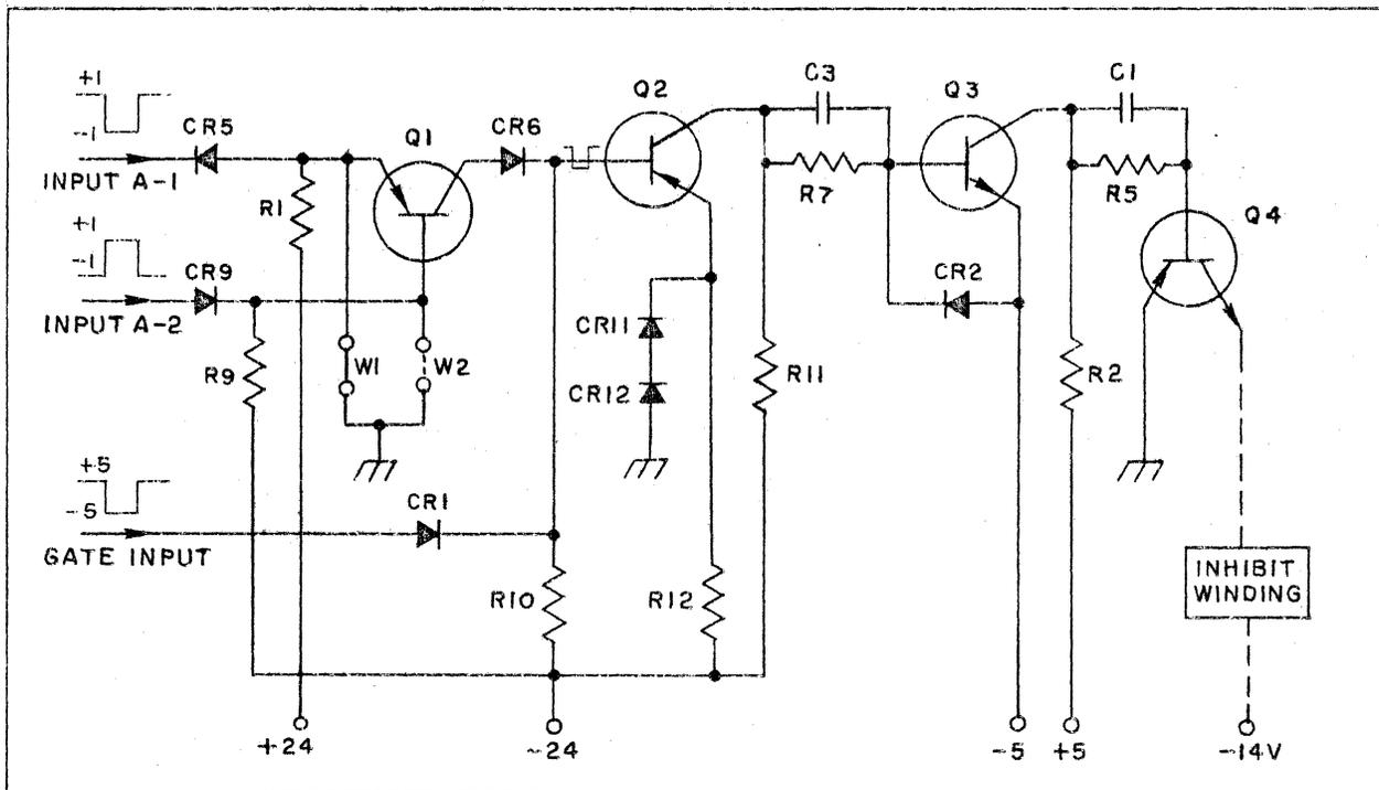
Figure 4-7. Digit Driver, Simplified Schematic Diagram
