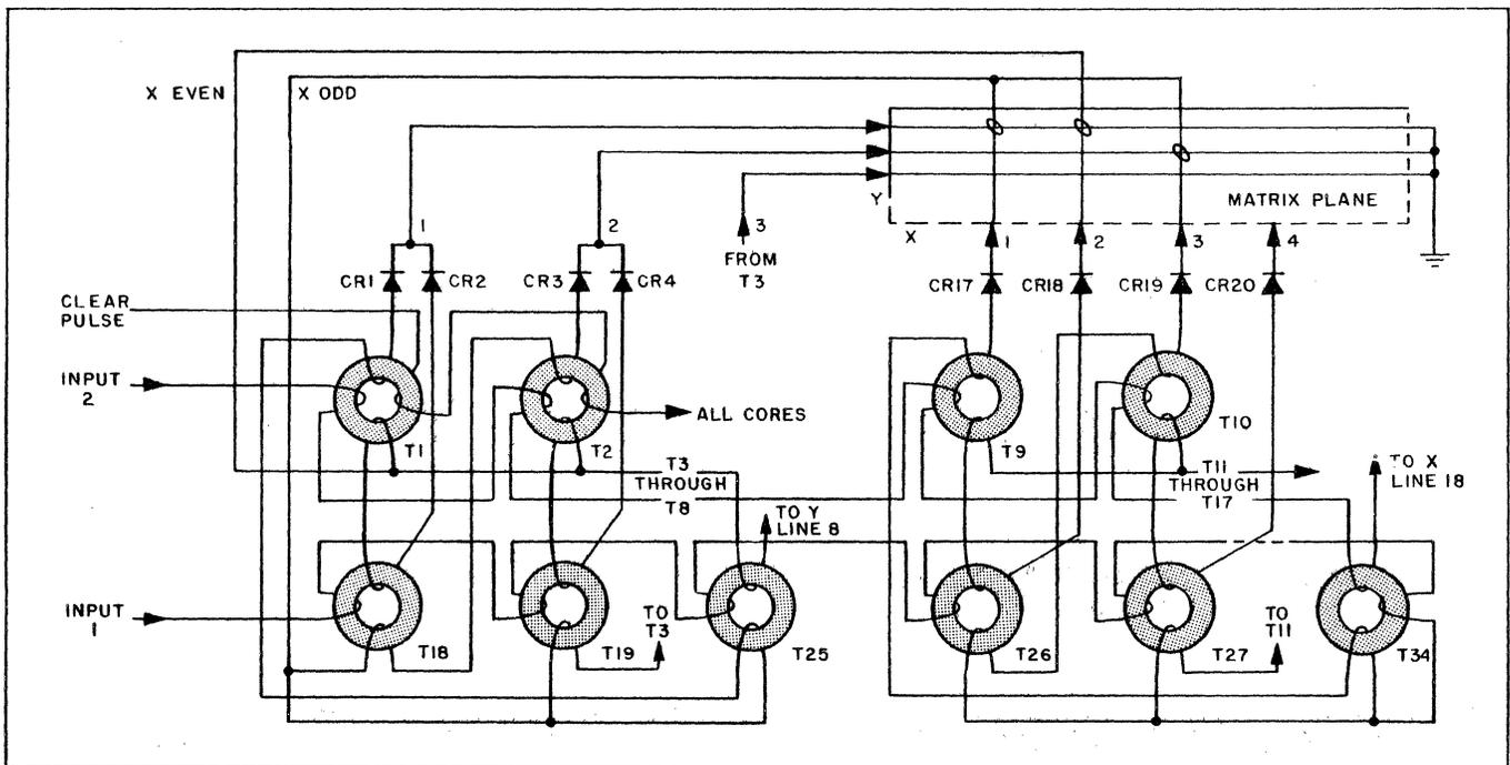
Figure 4-6. Magnetic Stepping Switches, Simplified Schematic Diagram
