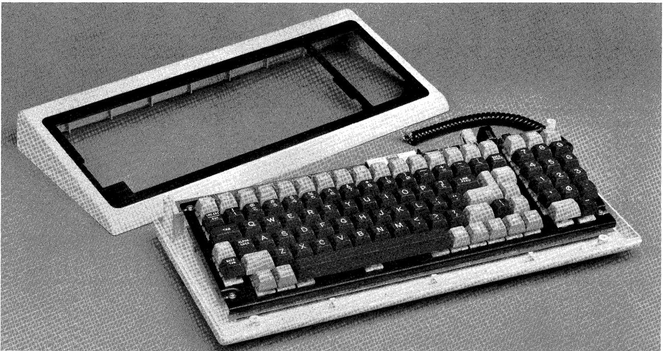
Keyboard cover removed for inspection.
