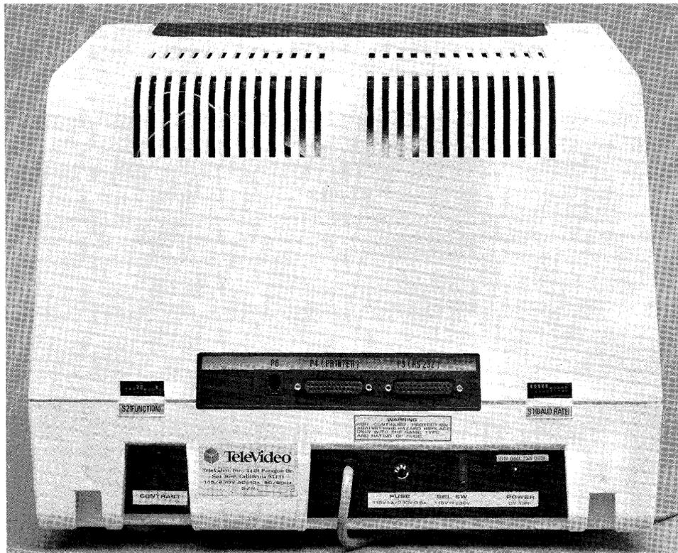
Figure 3-1 Model 950 Rear Panel Controls and Connectors
