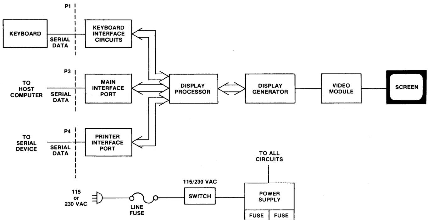
Figure 5-1 Model 950 Simplified Block Diagram
