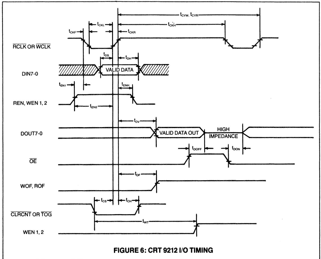
**FIGURE 6: CRT 9212 I/O TIMING**
