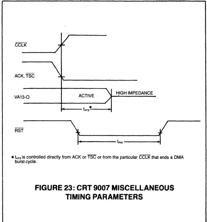
FIGURE 23: CRT 9007 MISCELLANEOUS TIMING PARAMETERS
