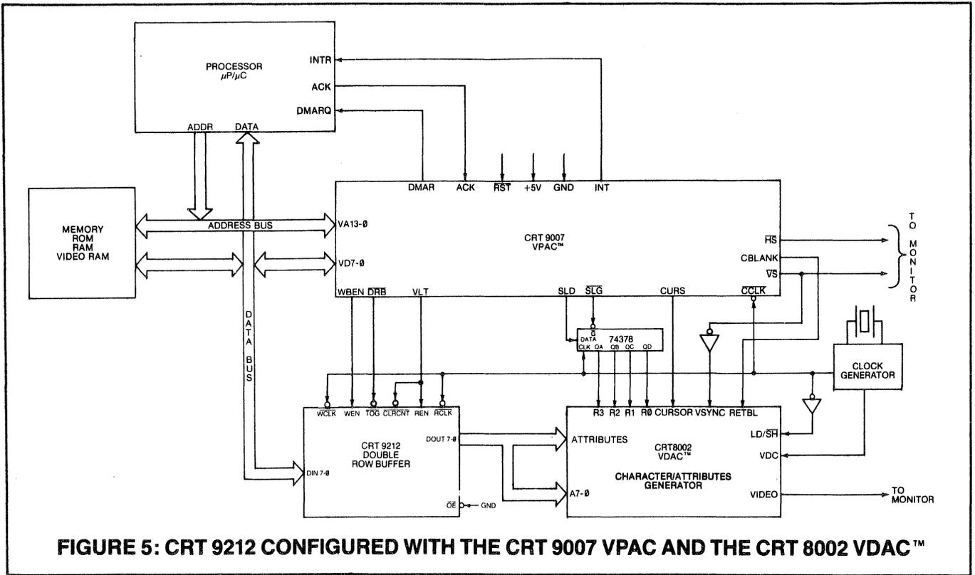
**FIGURE 5: CRT 9212 CONFIGURED WITH THE CRT 9007 VPAC™ AND THE CRT 8002 VDAC™**
