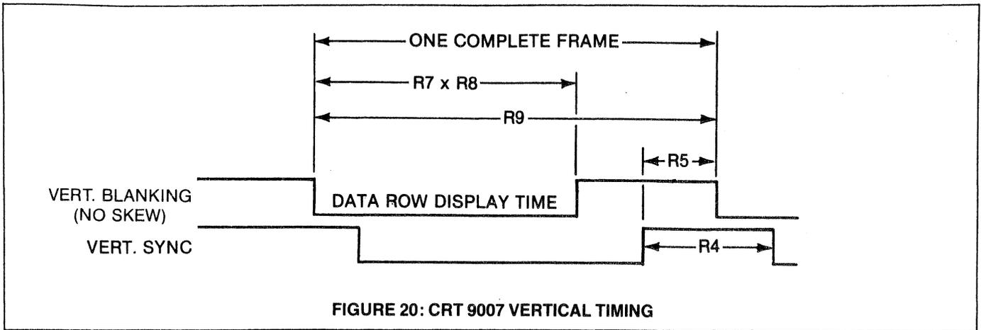
FIGURE 20: CRT 9007 VERTICAL TIMING
