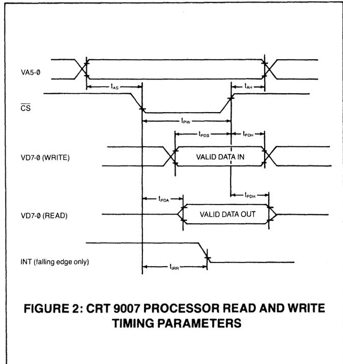
FIGURE 2: CRT 9007 PROCESSOR READ AND WRITE TIMING PARAMETERS
