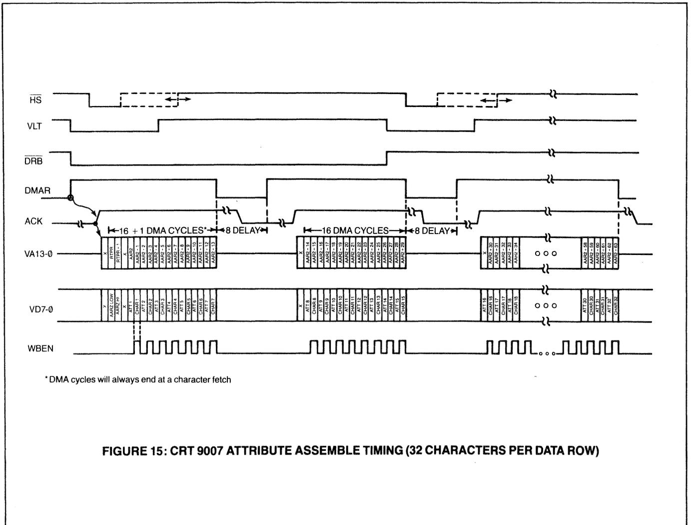
FIGURE 15: CRT 9007 ATTRIBUTE ASSEMBLE TIMING (32 CHARACTERS PER DATA ROW)
