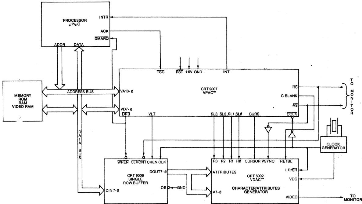
**FIGURE 6: CRT 9007 CONFIGURATION WITH SINGLE ROW BUFFER**
