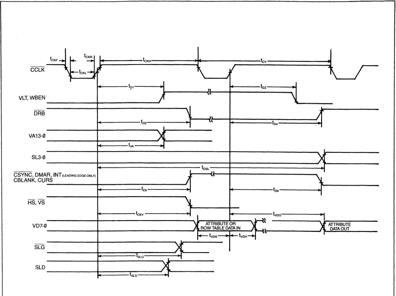
FIGURE 22: CRT 9007 TIMING PARAMETERS: OUTPUT SIGNALS
