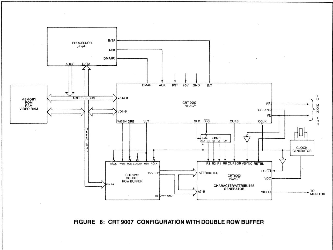
FIGURE 8: CRT 9007 CONFIGURATION WITH DOUBLE ROW BUFFER
