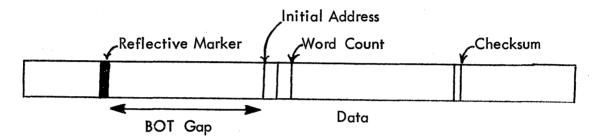
The initial address and word count are used by the READ routine to load the program without the necessity of any switch operations.
