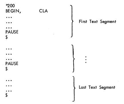
It is often convenient to use Tracks 1, 2, 3, and 4 of the same cartridge for text for a long program. More than one cartridge may be used if necessary.
