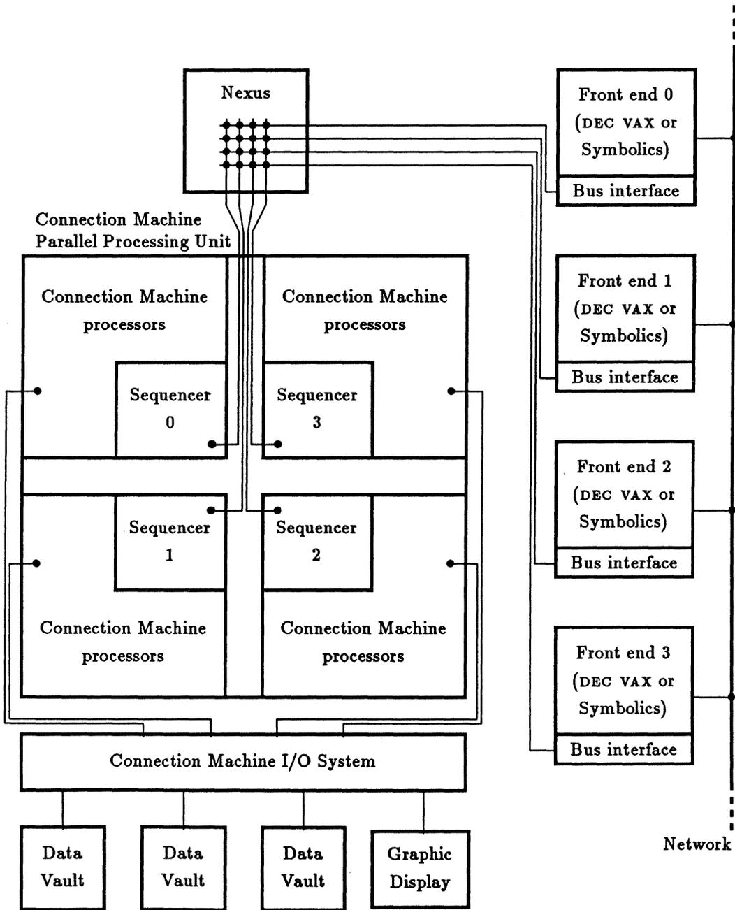
Figure 1: Connection Machine Model CM-2 System Organization
