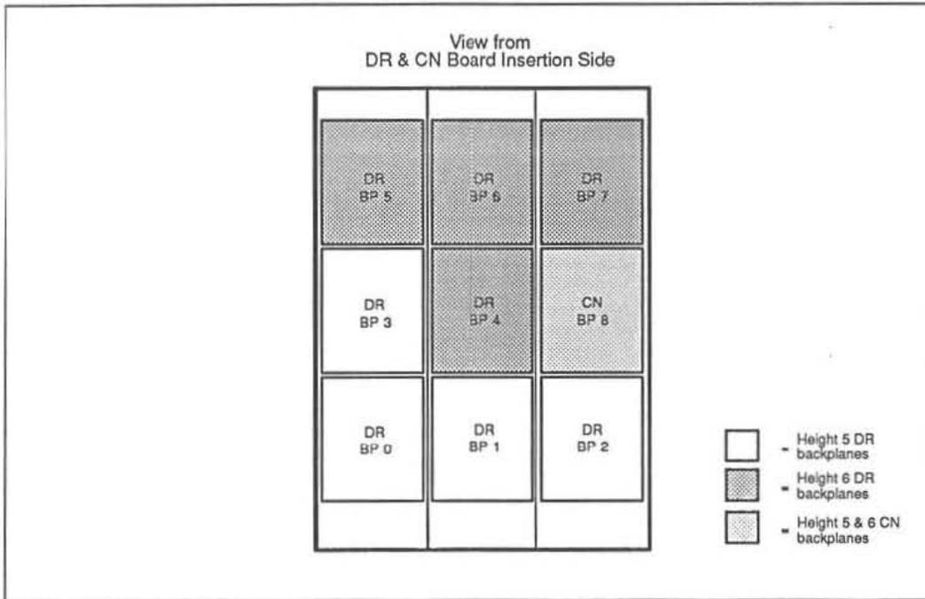
Figure 38. CM-5 network cabinets 0 and 1 backplane numbering
