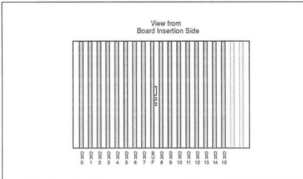
Figure 39. DR backplane slot assignments for network cabinets 0 and 1
