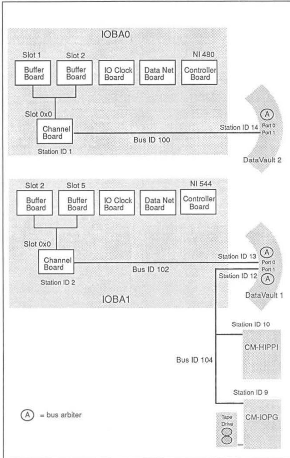
Figure 41. Sample CM-5 I/O system configuration.
