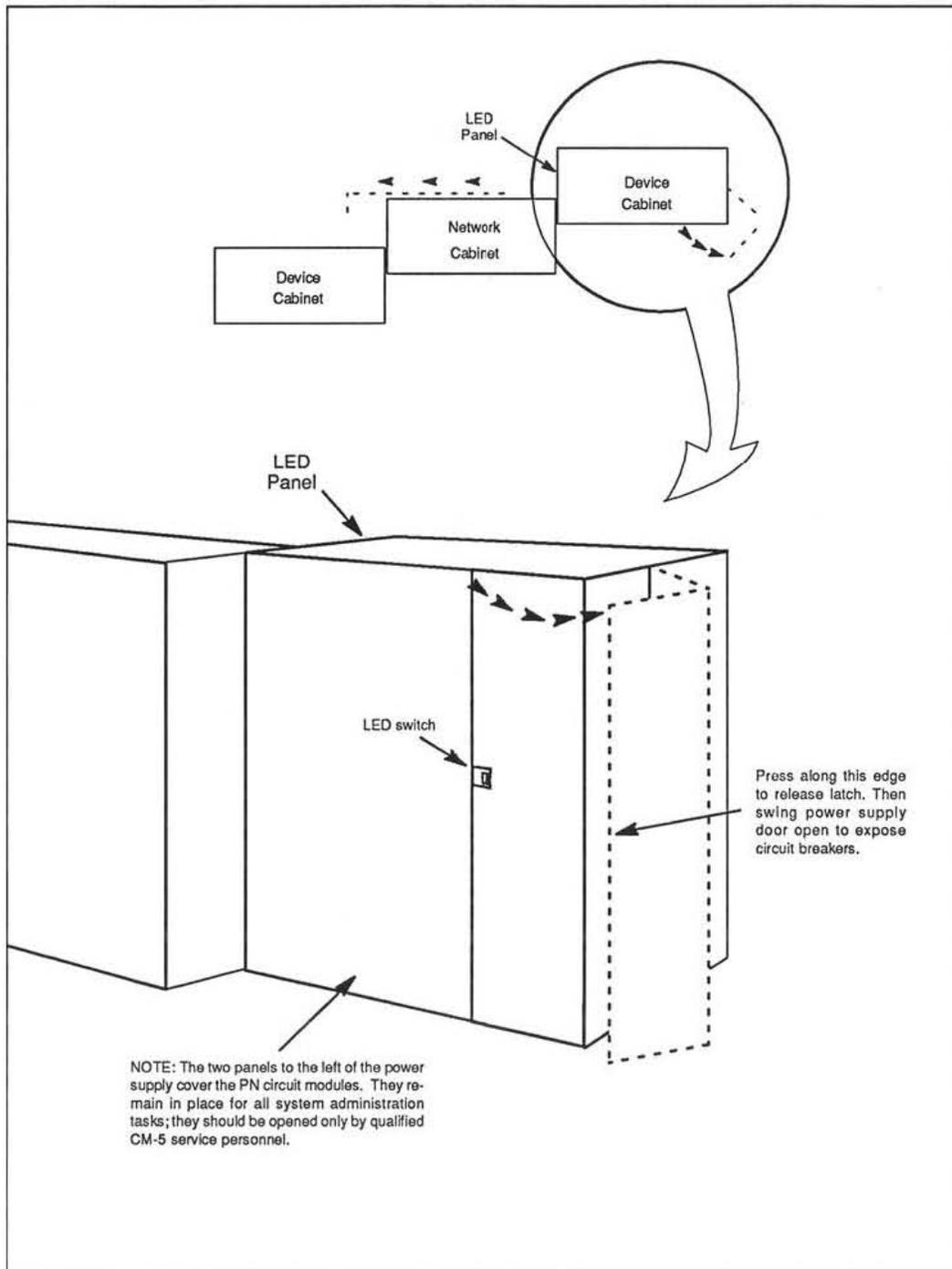
Figure 9. Access to device cabinet circuit breakers.
