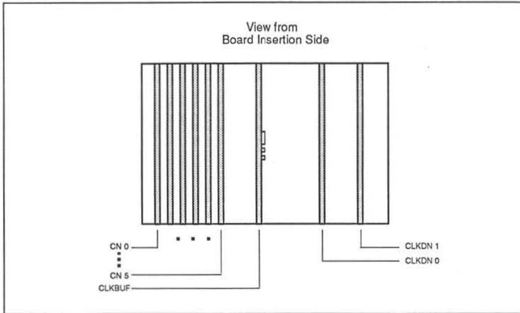
Figure 36. Device cabinet CN backplane slot assignments (backplane 10)
