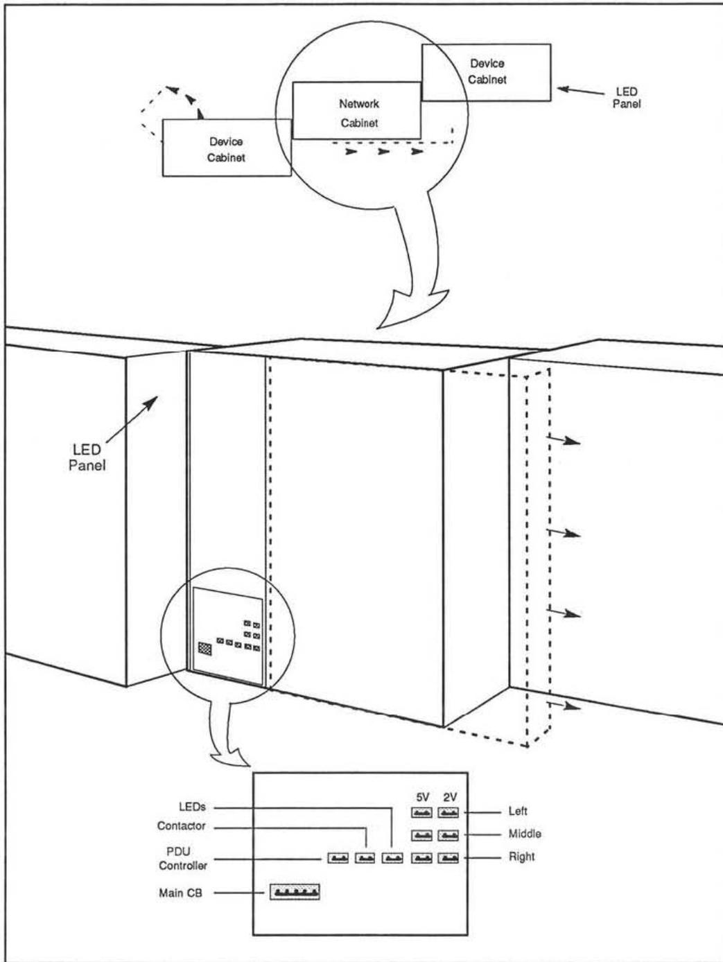
Figure 10. Access to network cabinet circuit breakers.
