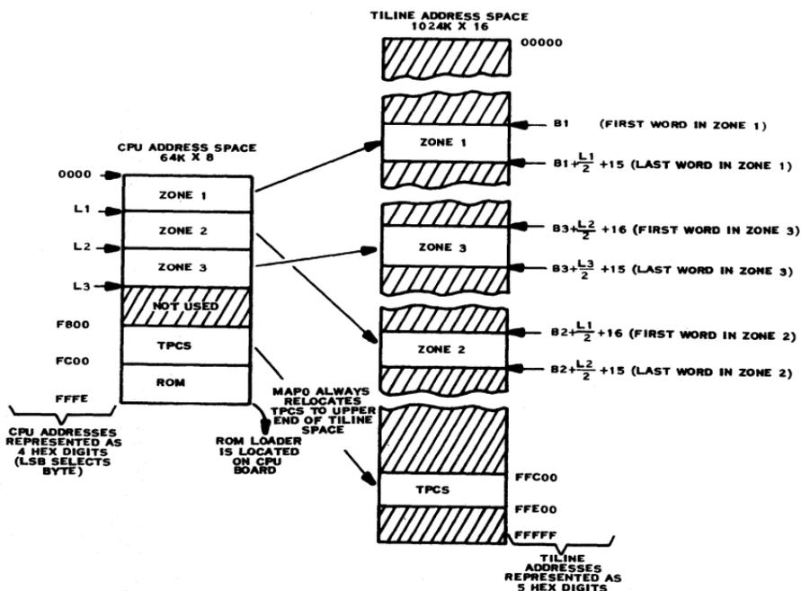
Figure 2-13. 990/10 CPU-TILINE Address Space with Map Option
