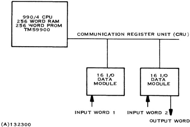
Figure 6-2. Hardwired Controller Block Diagram
