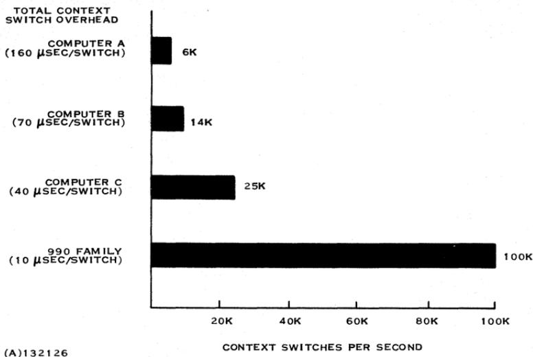
Figure 3-3. Comparison of Context Switching Efficiency
