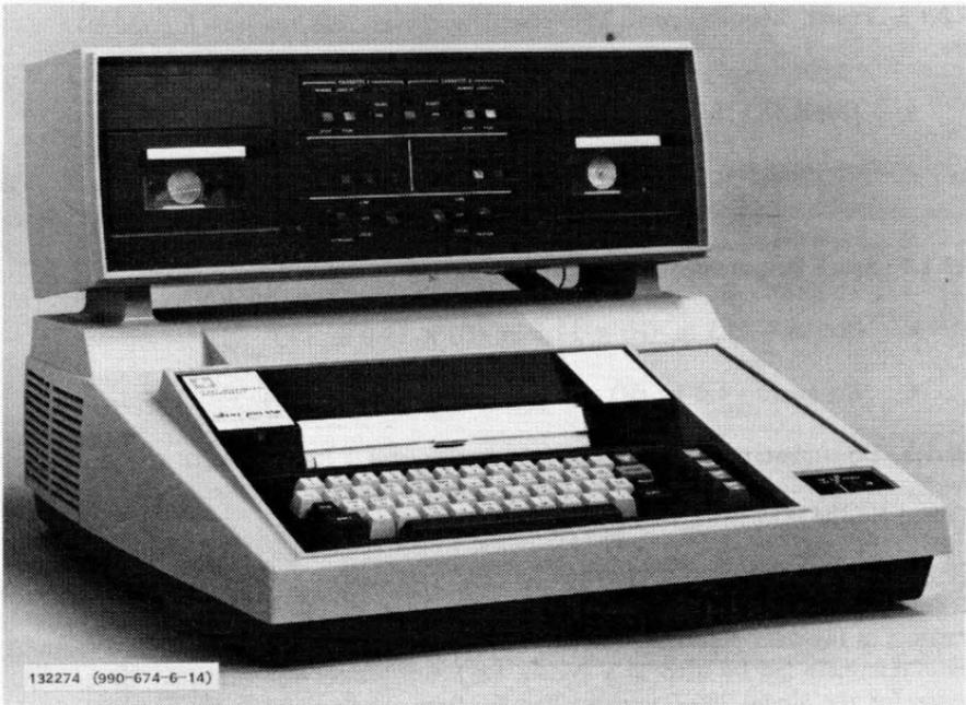
Figure 5-4. Model 733 ASR Data Terminal
