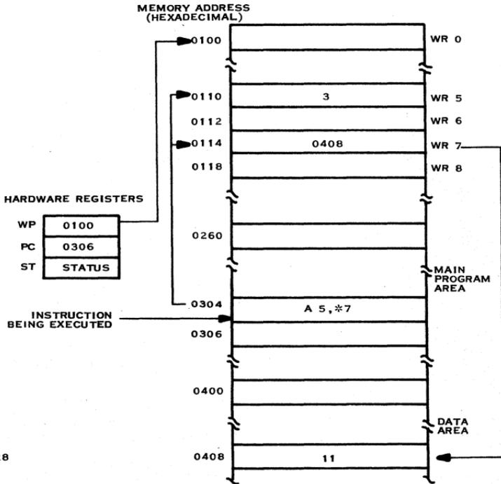
Figure 3-6. Indirect Workspace Register Addressing
