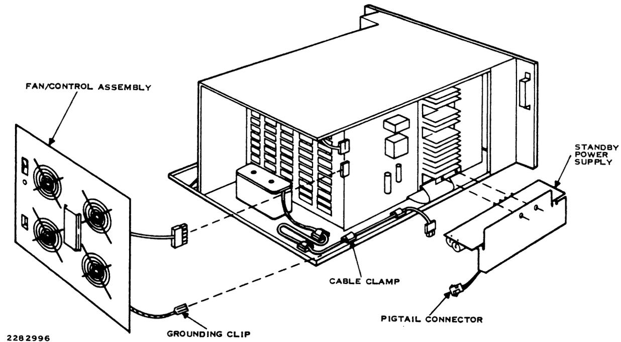
**Figure A-2. Battery Cable Clamp Locations**
