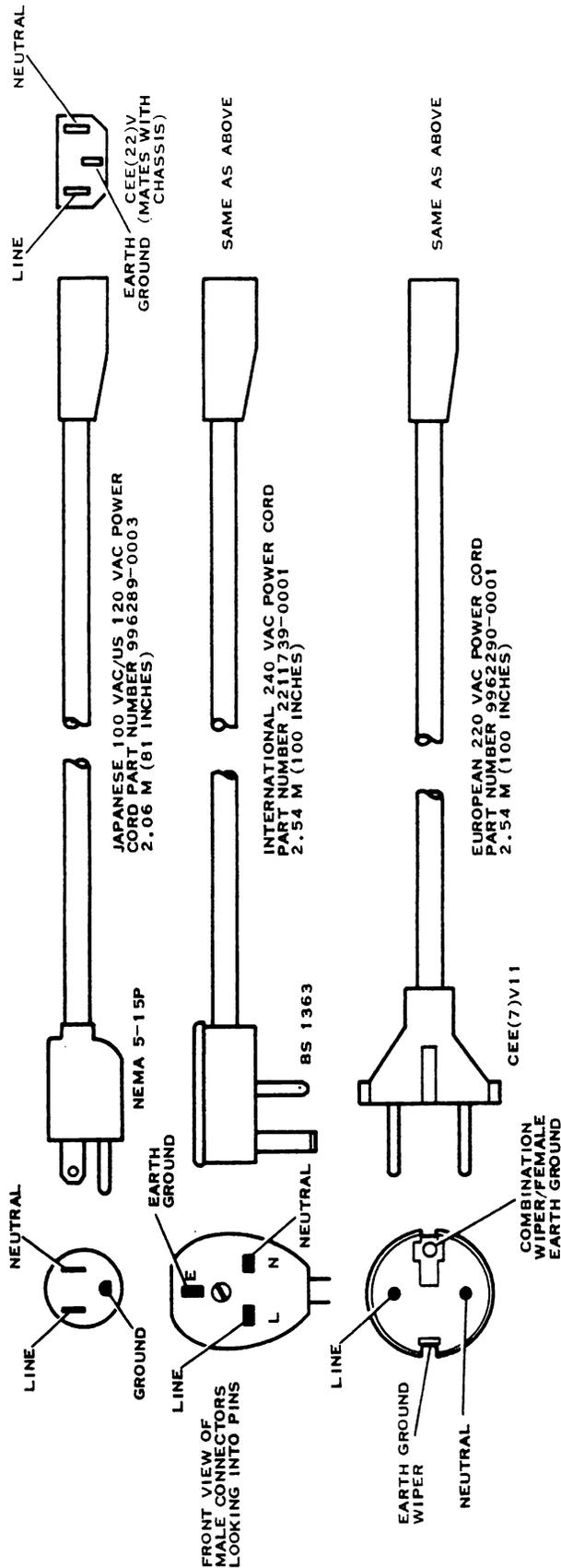
Figure 2-1. Power Cord Sets and Connectors
