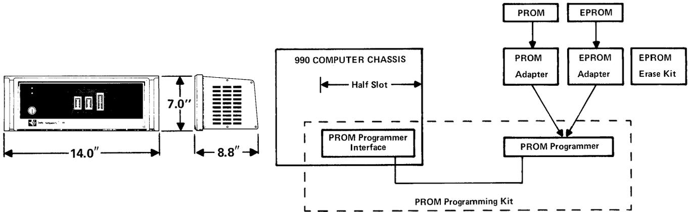
The PROM Programming Adapter plugs into the PROM Programmer and programs SN74S287, 471, and 472 devices.
