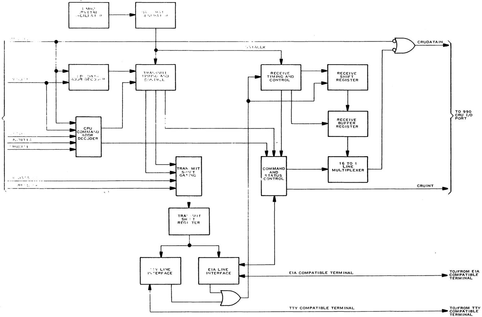
Figure 1-2. Full Duplex TTY/EIA Terminal Interface Module, Simplified Block Diagram
