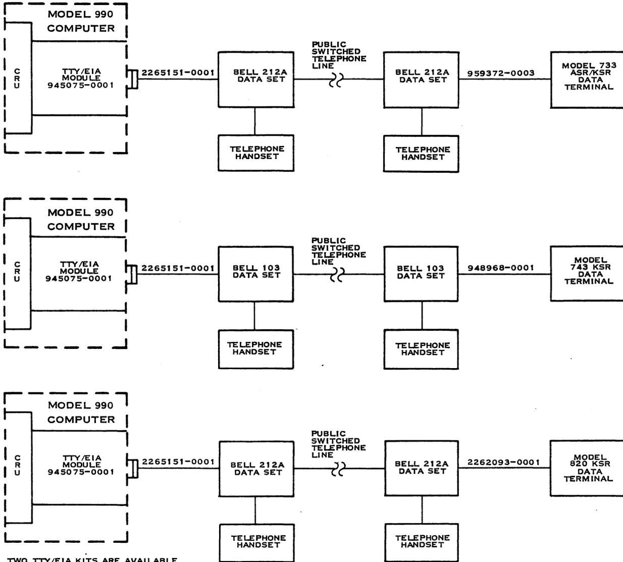
TWO TTY/EIA KITS ARE AVAILABLE, 2265150-0001 FOR 300 BAUD OPERATION OR 2265150-0002 FOR 1200 BAUD OPERATION. BOTH INCLUDE THE TTY/EIA MODULE AND THE MODEM CABLE.
