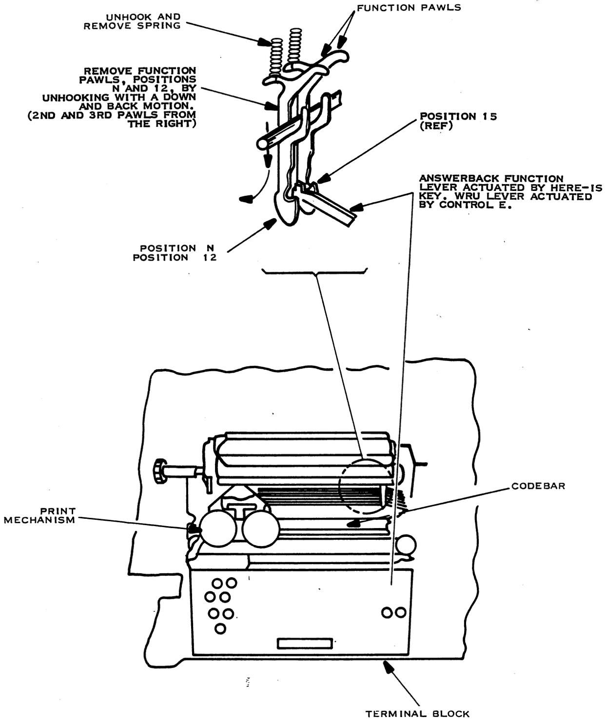
Figure 2-11. Answerback and WRU Function Bar Removal
