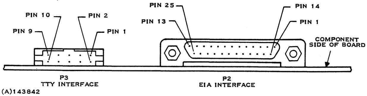
**Figure 2-2. TTY and EIA Connector Pin Numbering**
