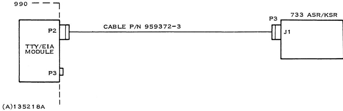
Figure 2-5. 990 Computer/733 ASR/KSR Interface, Cable Interconnection
