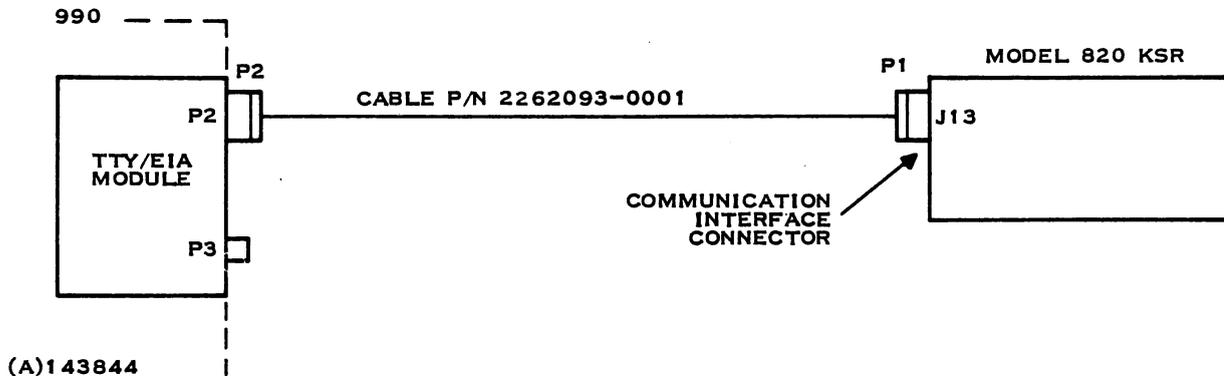
Figure 2-8. 990 Computer/820 KSR Interface, Cable Interconnection
