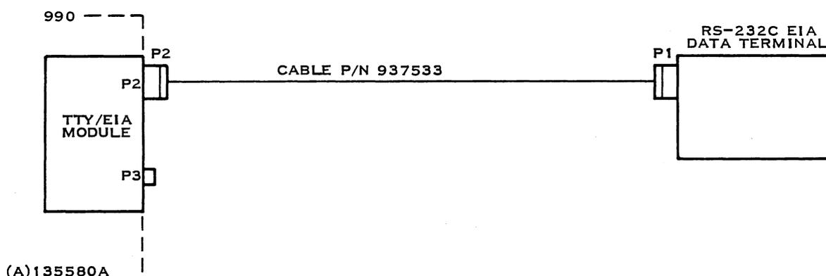
Figure 2-12. 990 Computer/RS-232C EIA Data Terminal Interface, Cable Interconnection
