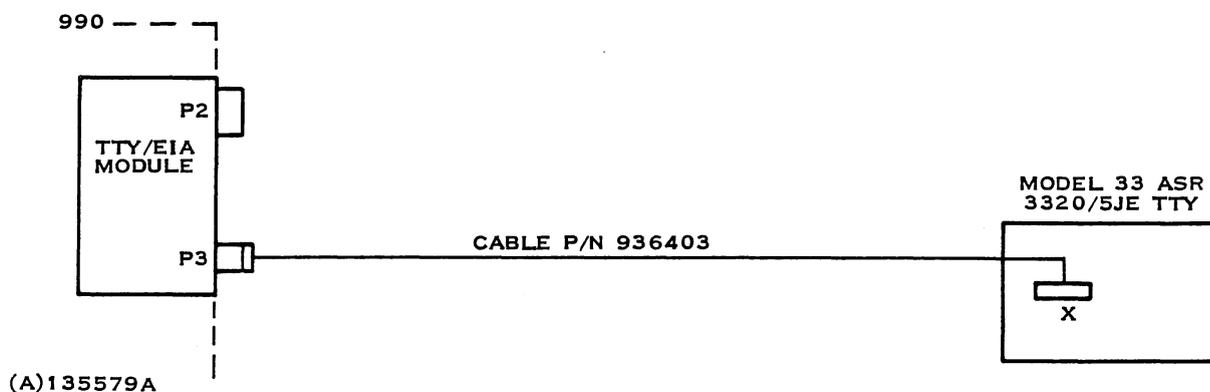
**Figure 2-9. 990 Computer/Model 33 ASR Interface, Cable Interconnection**
