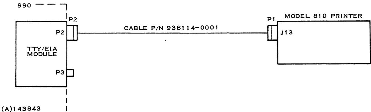
Figure 2-7. 990 Computer/810 Printer Interface, Cable Interconnection
