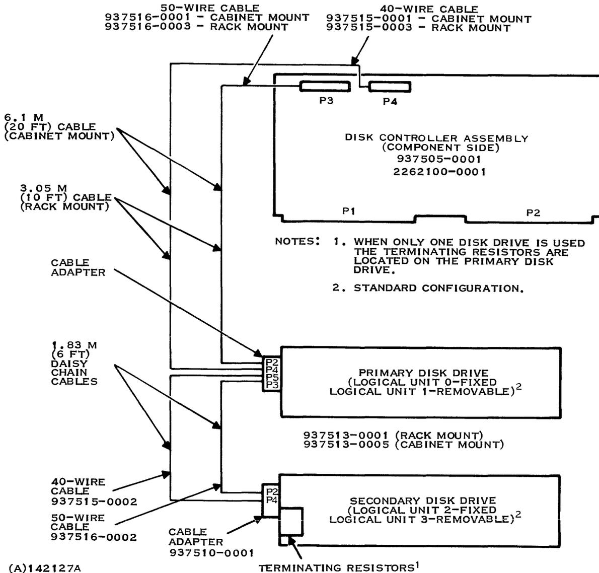
Figure 1-5. Interconnection of Disk Controller and Two Disk Drives
