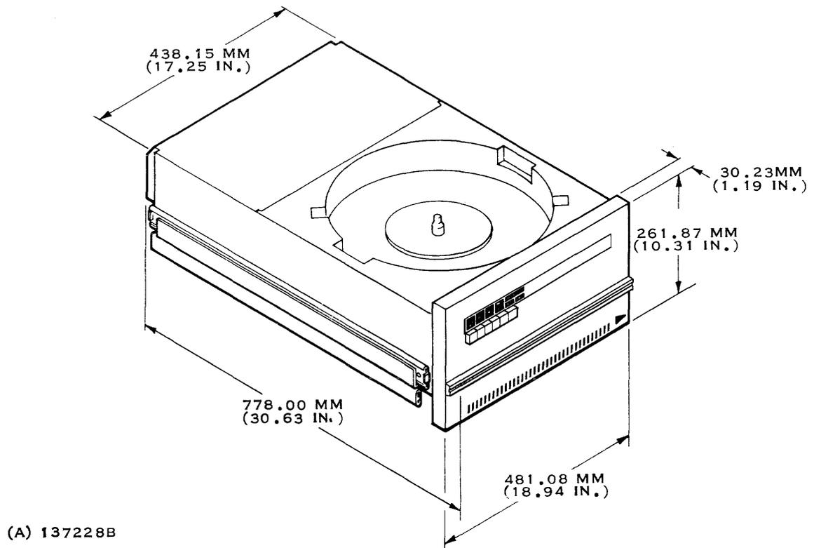
Figure 1-9. Rack Mount Disk Drive Physical Dimensions
