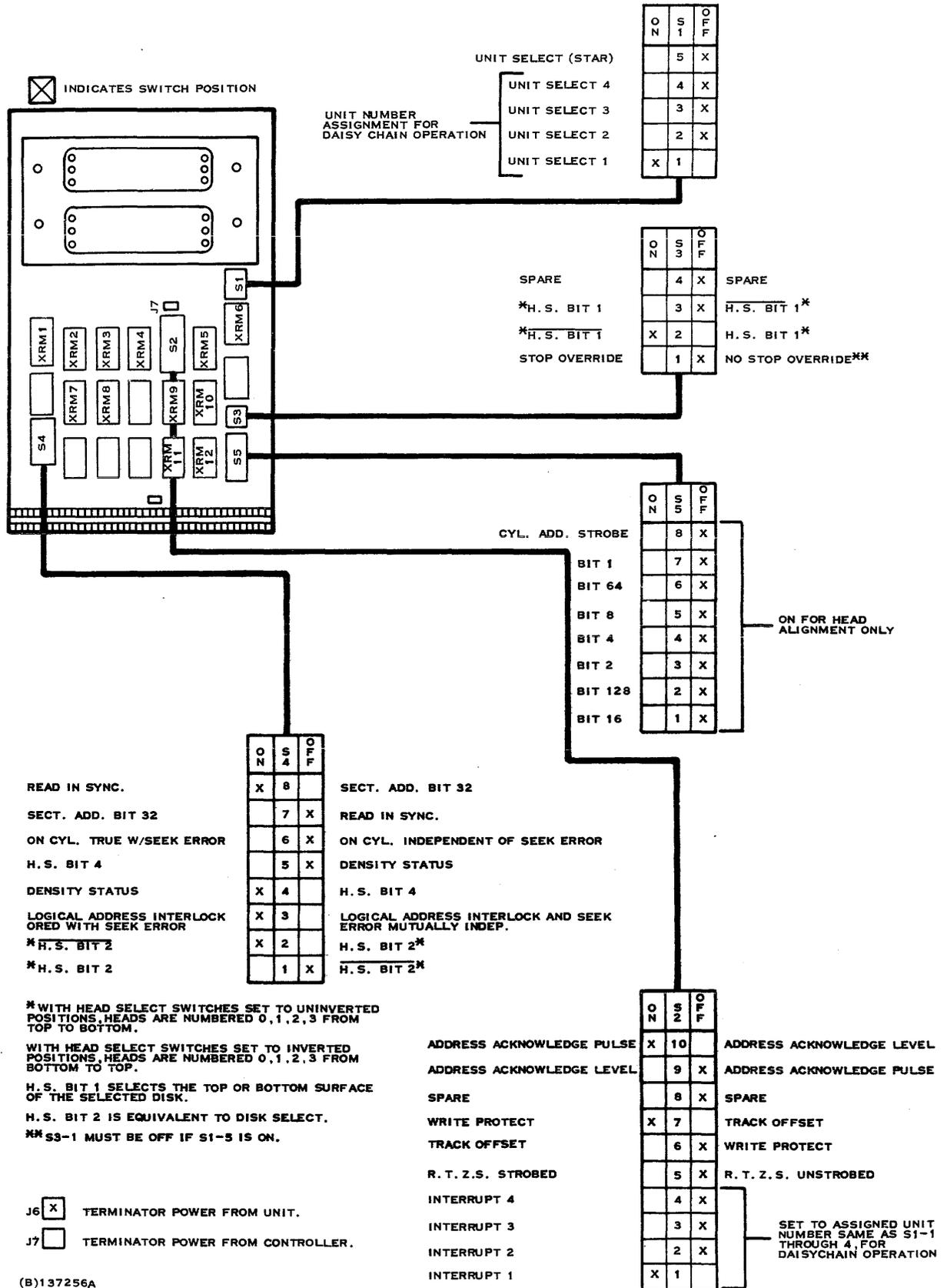
Figure 2-39. Switches and Settings for Rack Mount Primary Disk Drive
