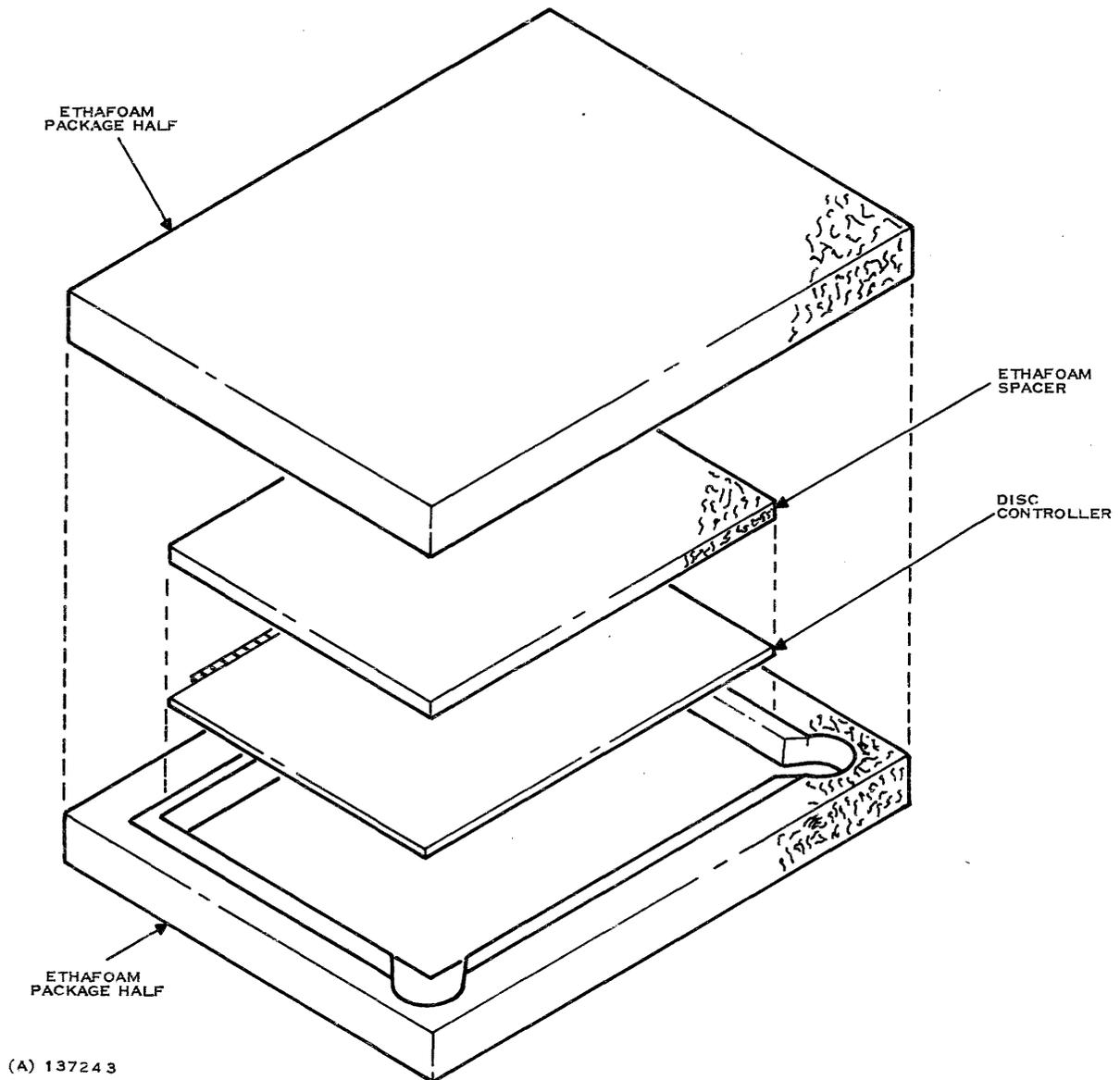
Figure 2-16. Disk Controller Shipping Configuration
