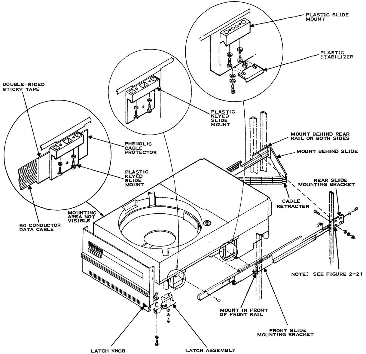
NOTE: THE TAPPED ANGLE ASSEMBLIES (973712-0006 FOR 1778 MM (70 IN.) RACK, 946738-0010 FOR 762 MM (30 IN.) RACK) AND THE CABLE CARRIER 996745-0001 ARE SUPPLIED WHEN DISK IS PURCHASED AS PART OF A DS990 KIT.
