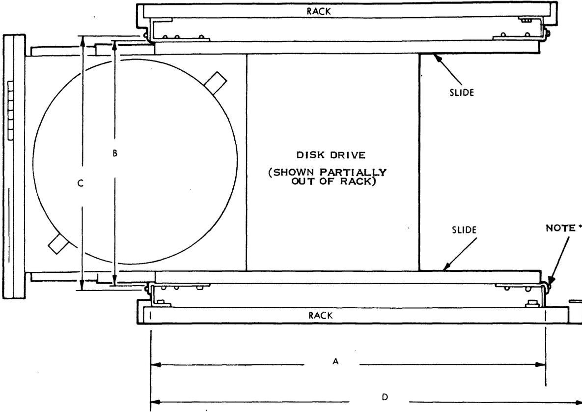
NOTE \* IF THE DRIVE IS MOUNTED IN A CABINET WITH A COMPUTER CHASSIS THE DIMENSION FOR "A" IS 622.3 MILLIMETERS (24.5 INCHES). THIS DIMENSION CAN BE ACCOMPLISHED BY REVERSING ONE OF THE SLIDE MOUNTING BRACKETS. (SEE FIGURE 2-21)
