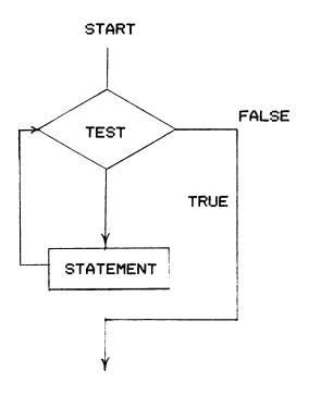
\*\*NOTE: THE VARIABLE CONTROLLING THE LOOP MUST BE MODIFIED IN THE STATEMENT TO AVOID AN INFINITE LOOP.
