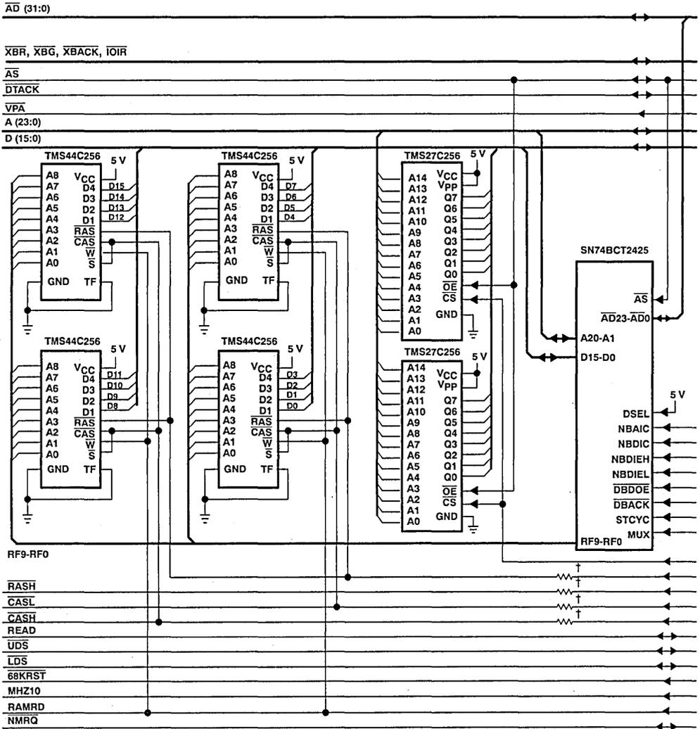
† Series damping resistors are recommended but may not be required, depending upon the system.
