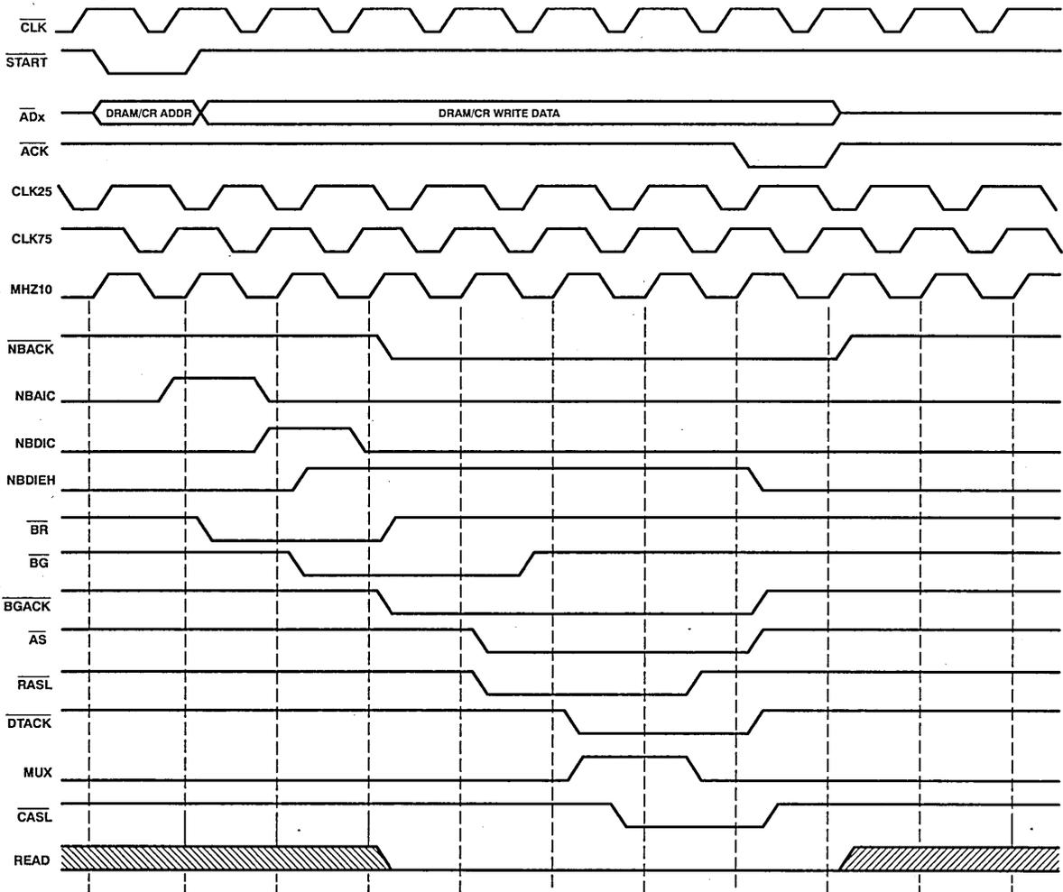
Figure 21. 8-Bit NuBus™ DRAM/CR Write Cycle
