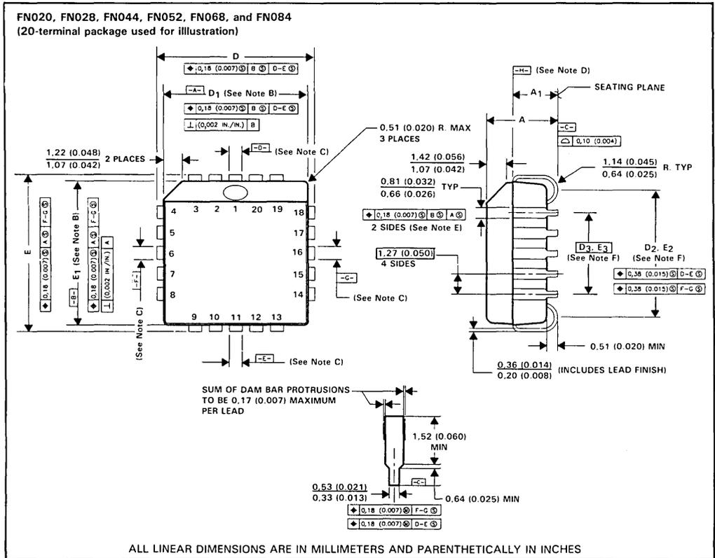
NOTES: A. All dimensions conform to JEDEC Specification MO-047AA/AF. Dimensions and tolerancing are per ANSI Y14.5M-1982.
