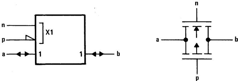
Figure 13. CMOS Transmission Gate Symbol and Schematic
