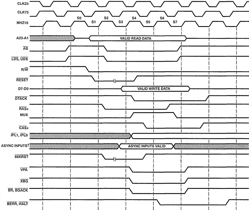
† The timing diagram assumes the asynchronous inputs FC1-FC0,  $\overline{BG}$ ,  $\overline{XBR}$ ,  $\overline{XBACK}$ , and  $\overline{IOIR}$  are recognized at the next falling CLK edge.
