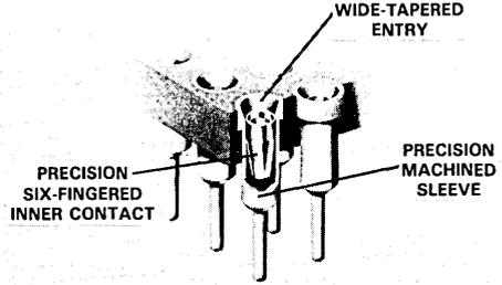
Inner contact - 30  $\mu$ m gold over 50  $\mu$ m nickel or 100  $\mu$ m tin/lead over 50  $\mu$ m nickel
