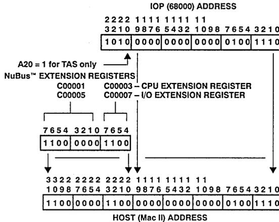
Figure 6. IOP (I/O Processor) to NuBus™ Address Translation
