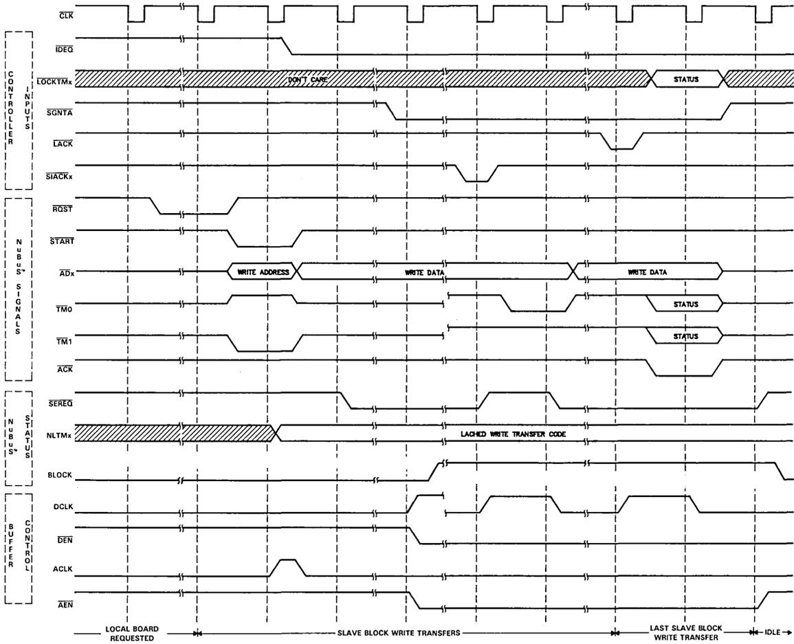
†The BLOCK signal must be supplied by external logic, such as from TI's SN74ALS2442.
