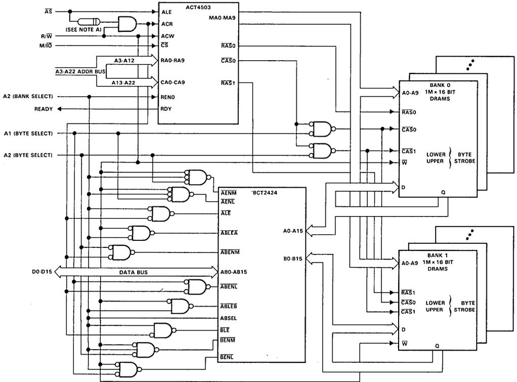
NOTE A: The value of this delay element is dependent on the speed of the microprocessor.
