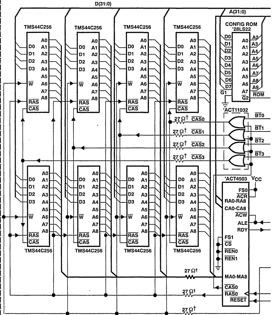
† Series damping resistors are recommended but may not be required, depending upon the system environment.
