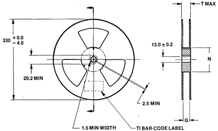
Variables are used in Figure 6 and Table 3. The definitions for the variables are as follows: G is the distance between the flanges, T is the maximum reel width, and N is the diameter of the reel hub. All dimensions are given in millimeters.
