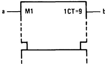
Figure 20. An Output of the Common-Control Block
