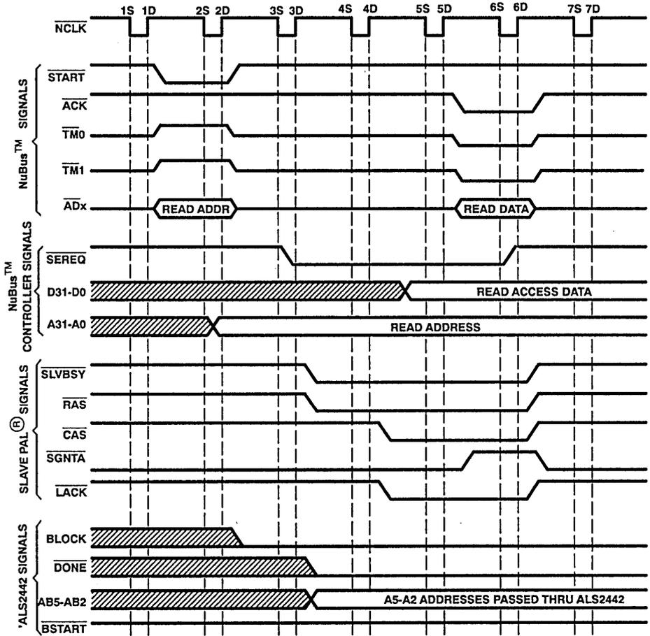
Figure 4. Normal (Nonblock) Read Cycle
