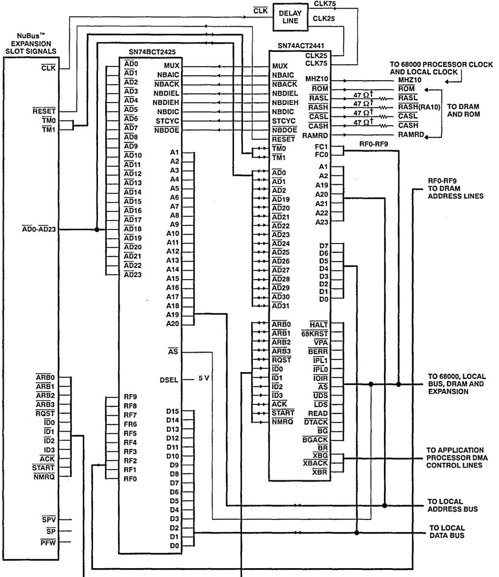
† Series damping resistors are recommended but may not be required, depending upon the system.
