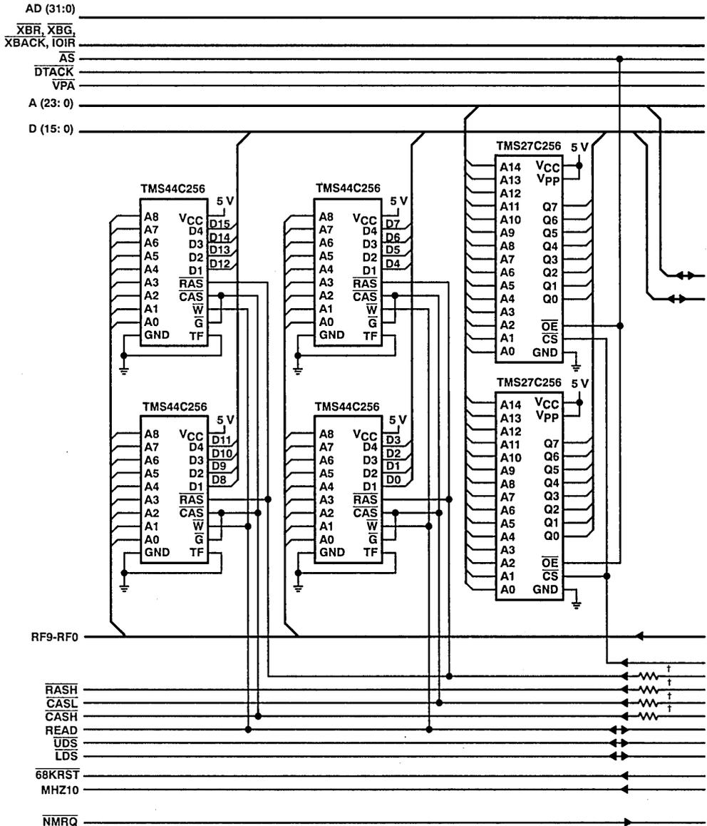
† Series damping resistors are recommended but may not be required depending on system environment.
