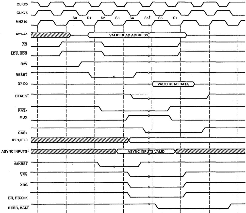
† During ROM read cycles, one wait state is inserted by the 'ACT2441 MCP controller via DTACK.
