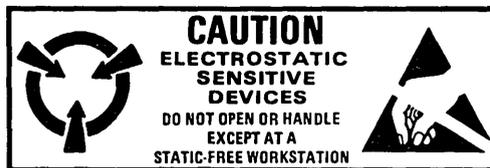
3. The warning label shall be legible and easily readable to normal vision at a distance of 3 feet.
