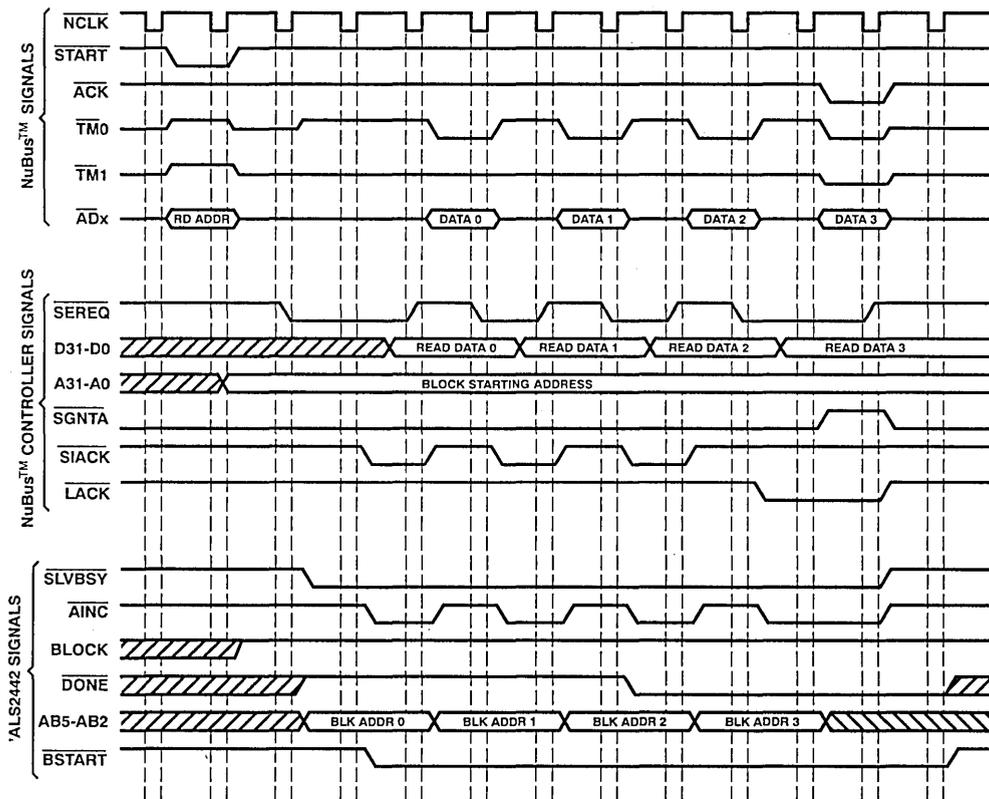
FIGURE 1. TYPICAL BLOCK READ TRANSFER (4 WORDS)
