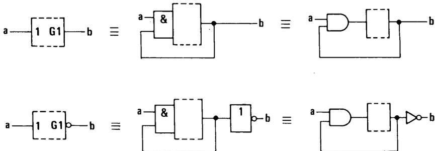
Figure 5. G Dependency Between Outputs and Inputs
