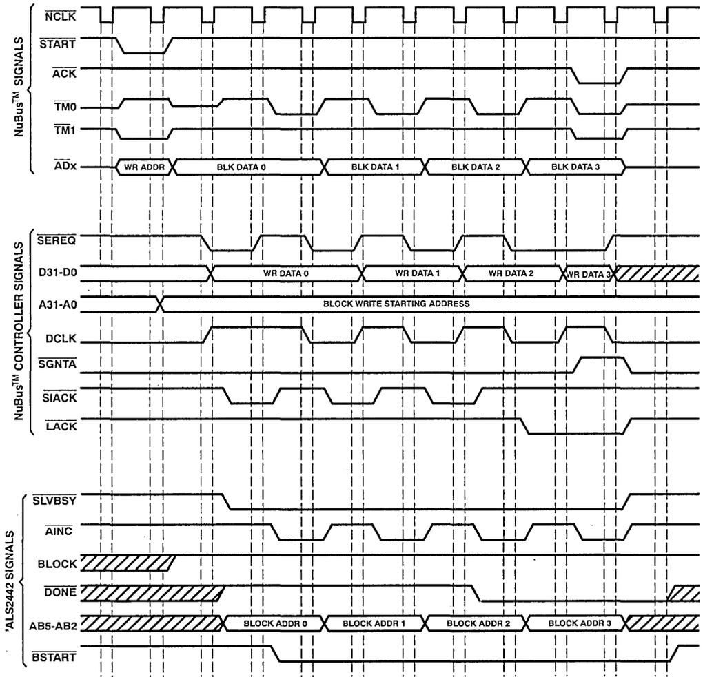
FIGURE 2. TYPICAL BLOCK WRITE TRANSFER (4 WORDS)
