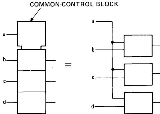
Figure 2. Common-Control Block
