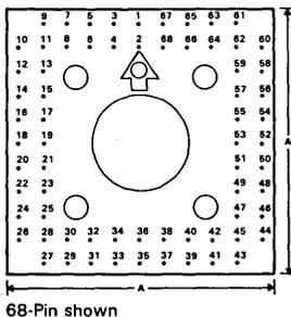
NOTE: Socket electrical pin-out pattern represents component side of P.C.B. layout. (TYP. counter clockwise numbering pin-out system.)
