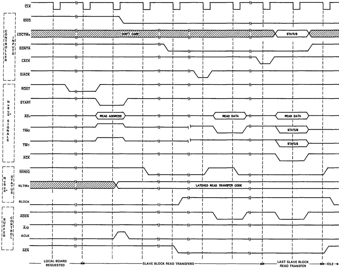
† The BLOCK signal must be supplied by external logic, such as from TI's SN74ALS2442.
