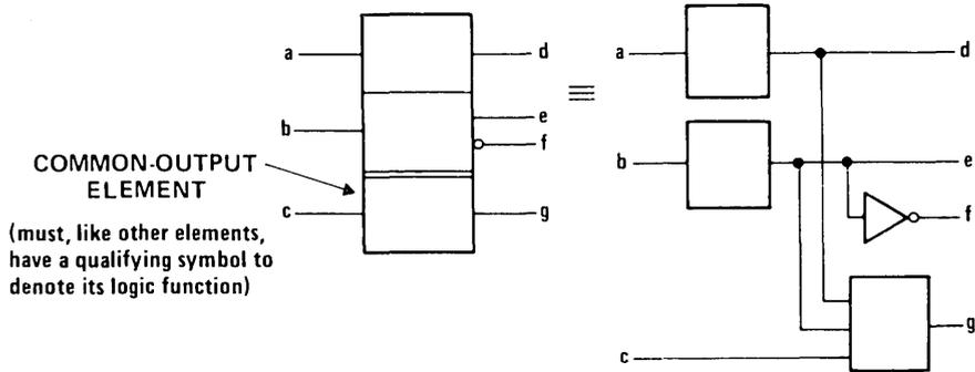
Figure 3. Common-Output Element
