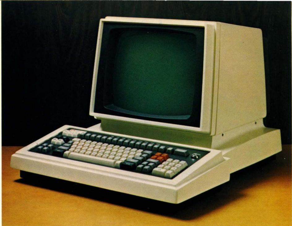
*The Model 914A Video Display Terminal is the basic CRT unit of DXS. The 914A is an intelligent terminal with its own operating system (down-loaded from the DXS terminal monitor). Much of the editing of data is done by the terminal.*
