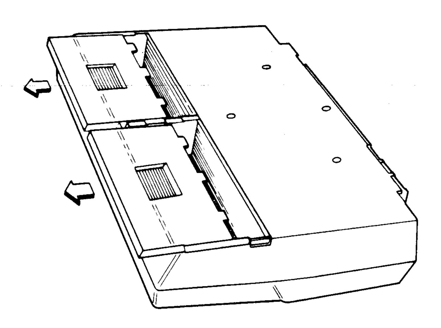
3. Connect the connector of each battery unit to the connector in each battery compartment.
