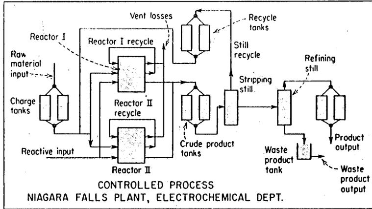
Fig. 11. Controlled Process
