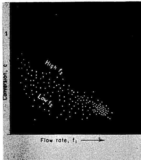
FIG. 3. Conversion as a function of flow rate  $f_1$ , shows effects of catalyst flow rate  $f_2$ .
