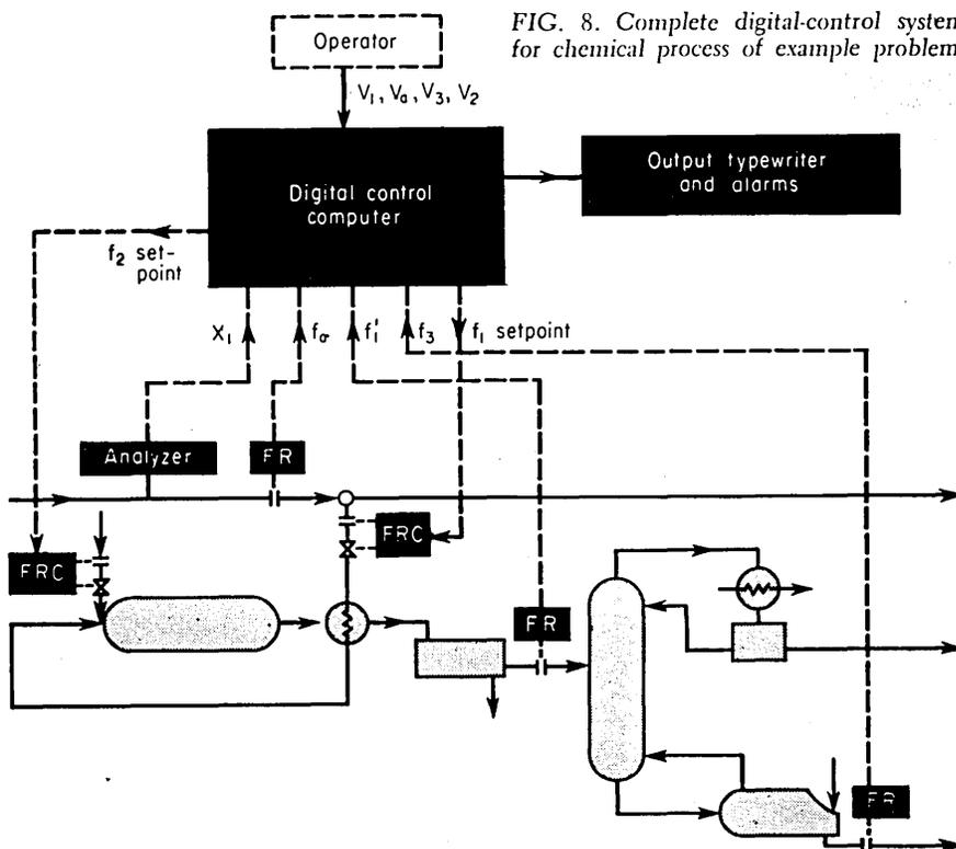
FIG. 8. Complete digital-control system for chemical process of example problem.
