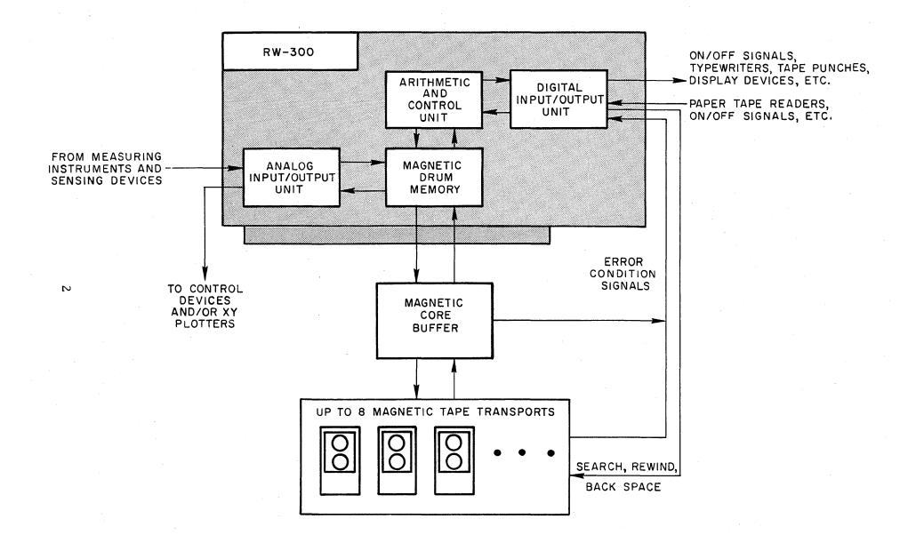
facilitate broad communication with physical phenomena and human operators. In addition, the RW-300 offers full general-purpose computing abilities.
