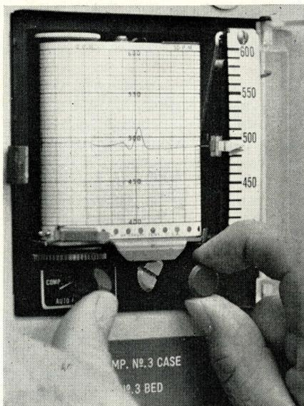
**RECORDER CONTROLLERS** can be set by hand, or directed by computer. Bump in chart shows effects of feed change.
