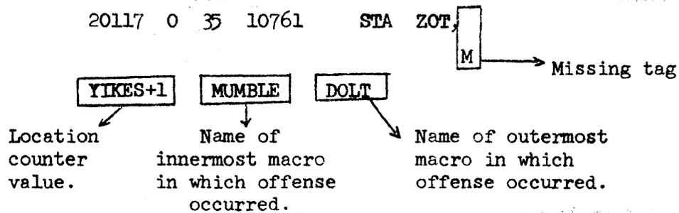
Thus along with each error the location counter is printed out relative to the symbol most recently defined. In addition, if the error occurs during macro expansion the names of the innermost and outermost macros are printed to give a clue on where to look for the error. If only one level of macro expansion is involved, then only that name is listed.
