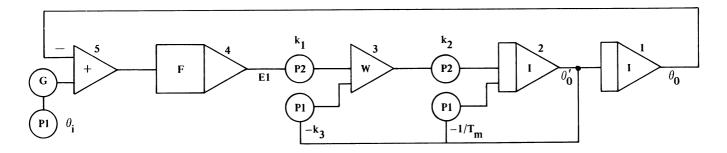
Of special importance in this example is the use of the function generator to describe the output of the amplifier. The gain of the amplifier is proportional to the position error  $(\epsilon)$  such that:
