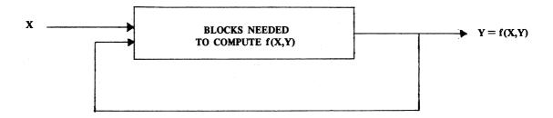
This configuration contains an algebraic loop and will give a sort failure error message. However, the wye and vacuous blocks may be used to accommodate this algebraic loop as discussed above.
