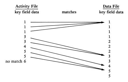
The SINGLE option instructs UPDATE to use only the first of several matching activity records to update a data record. If other data and activity records contain the same key field data, the process is repeated. The diagram below illustrates the matching procedure in UPDATE when the SINGLE option is requested.<sup>1</sup>
