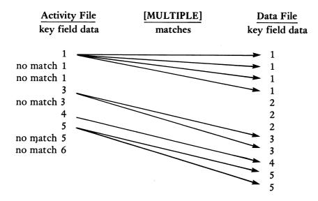
The UPDATE [MULTIPLE] matching procedure is the same as the normal matching procedure for SELECT, PURGE, and REPLACE.
