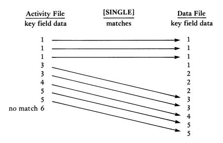
The MULTIPLE option provides an alternative method for matching data and activity records in the UPDATE procedure. Normally all activity records which specify the same key field data are used to update the first matching data record. When the MULTIPLE option is specified, a single activity record is used to update all data records that specify the same key field data. The following diagram illustrates the matching procedure in UPDATE when the MULTIPLE option is specified.
