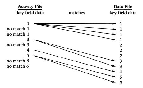
The SINGLE option in REPLACE, SELECT, and PURGE instructs IML to match an activity record with only the first unused data record which specifies the same key field data. The diagram below illustrates the matching procedure in REPLACE, SELECT, or PURGE when the SINGLE option is requested.<sup>1</sup>
