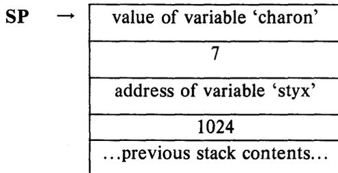
Functions are called by issuing either a "bsr" instruction or a "jsr" instruction, depending upon whether the callee is within a 16-bit addressing range or not, and whether the C optimizer was used. The "bsr" or "jsr" instruction pushes the return address upon the stack, and then branches to the indicated function. After the call, on entry to the function, the stack looks like this:
