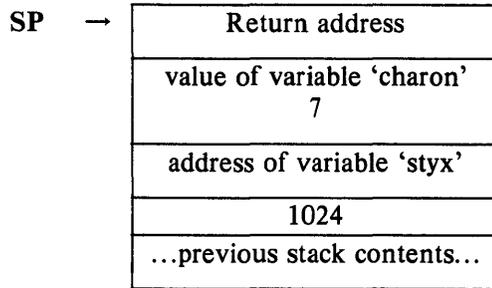
In each function, register A6 is used as a stack frame base. The stack location referenced by A6 contains the return address.
