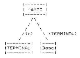
n is an integer MUMPS port number ( $\emptyset$ -6) TERMINAL is a terminal name like ADM3A Desc is a description of the terminal in the following format:
