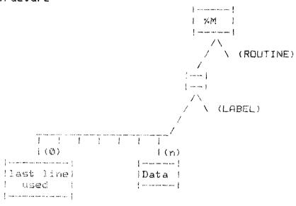
ROUTINE is a Routine name LABEL is a Routine line label last line used an integer pointing to the last data node (n) Data free text comments.
