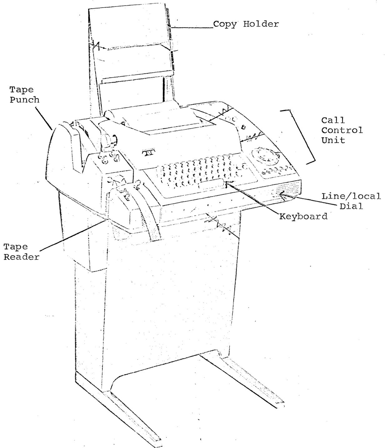
Figure 1. Automatic Send-Receiver (ASR) Teletypewriter Set
