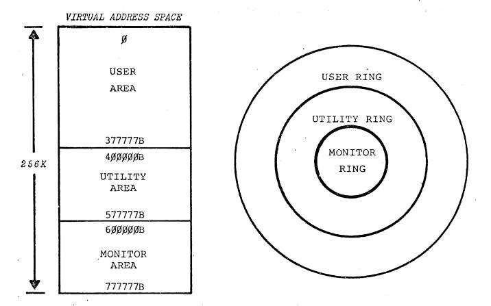
FIGURE 3.1 VIRTUAL ADDRESS SPACE AND PROTECTION RINGS
