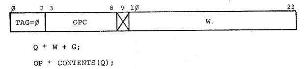
In the direct or G-relative mode, the effective address is given by the 14-bit address field relative to G. This permits direct addressing of the first 16K of the global environment. The notation in SPL is
