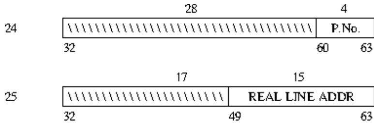
The normal virtual address format contains a segment number. Here the segment number is implied. It is the name segment of the process given by line 24. The line address in line 25 references a 64-bit word boundary in the name segment.
