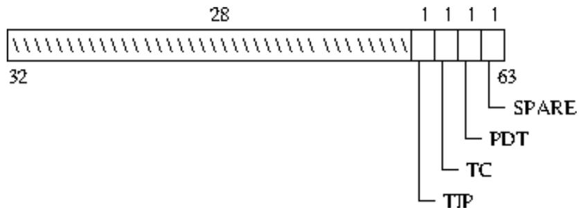
Bit 60 is the Transfer in Progress bit. Setting this bit initiates a block transfer. It may be reset by software to terminate the transfer midway. Hardware resets this bit on transfer complete (successful or not).
