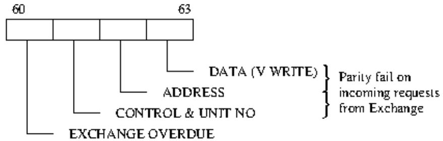
Writing to this line resets all bits and resets the l.s. 4 bits of Block 4 line 20.
