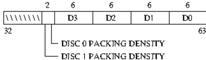
This line gives the current positions of each of the discs and also records which packing density is current ('0' = HALF P.D., '1' = FULL P.D.).
