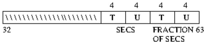
Seconds and fractions of seconds in b.c.d. as shown. This line is staticised by reading TIME.UPPER.
