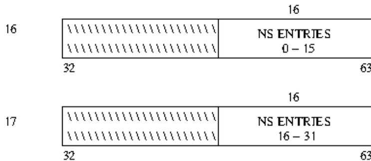
These lines have only READ access. However, writing to these addresses results in hardware action in the PROP V-store without disturbing NS LINE COPY.
