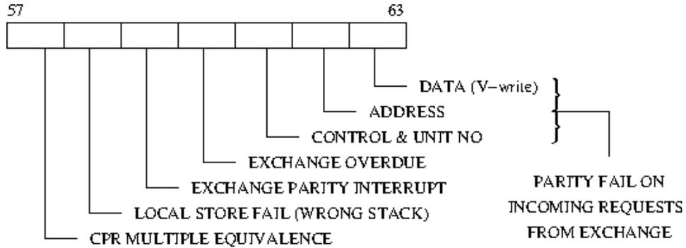
These bits are all set independently of on another, as their respective faults are detected. Writing to this line resets all bits except bit 58 and also resets line 20 and block 7 line 1. Bit 58 detects a hardware fault that cannot be cleared by software and can only be reset by general reset. General reset resets all bits. Writing to block 7 line 1 clears the bottom 4 bits
