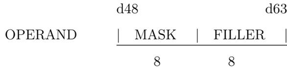
SMVB Moves one byte from source to destination. If the source string is a null string, move FILLER to destination. If DB = 0 there will be a BCH interrupt. Updates DO, DB, XDO, XDB.
