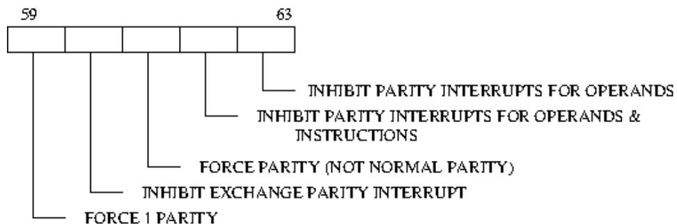
Interrupt inhibits do not inhibit the setting of the parity fail bits in lines 20 and 23. All bits in this line are cleared by general reset.
