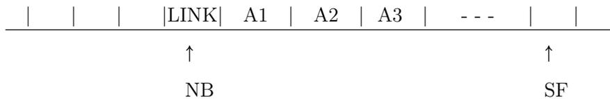
The RETURN will reset MS, NB, CO from the LINK in the store and return SF to its original position.
