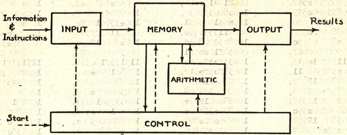
Figure 1--Basic Components of an Automatic Computer
