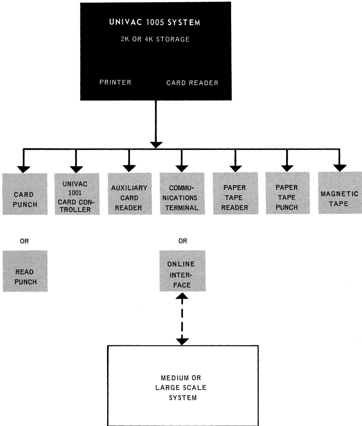
Figure 2-3. Maximum System Configuration
