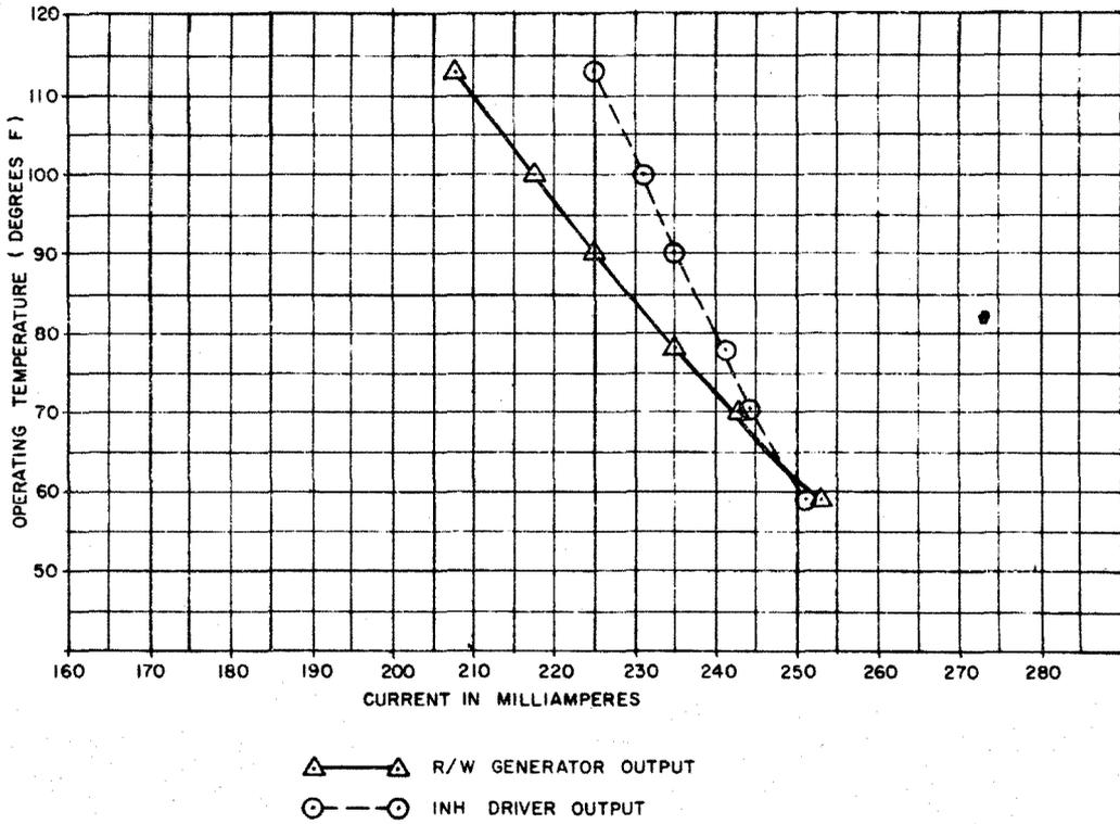
Figure 4-3c. Read/Write and Inhibit Current vs Temperature
