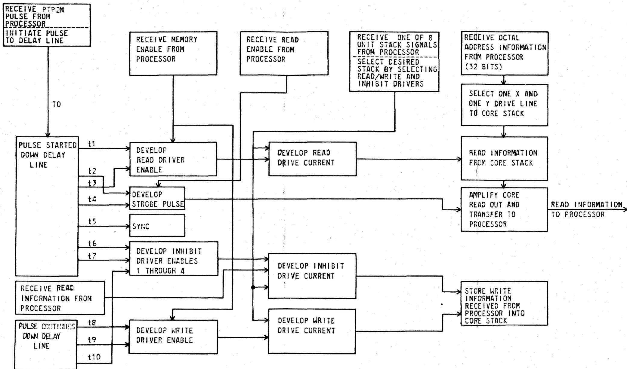
Figure 3-4. Timing Sequence of Read/Restore Cycle
