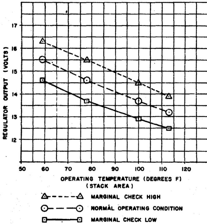
Figure 4-3a. Voltage Regulator Output vs Temperature
