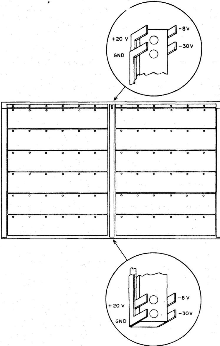
Figure 5-1. Rear View of Memory (Showing Voltage Terminals)
