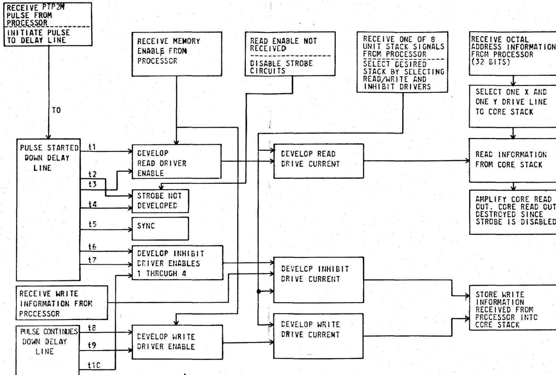
Figure 3-3. Timing Sequence of Clear/Write Cycle
