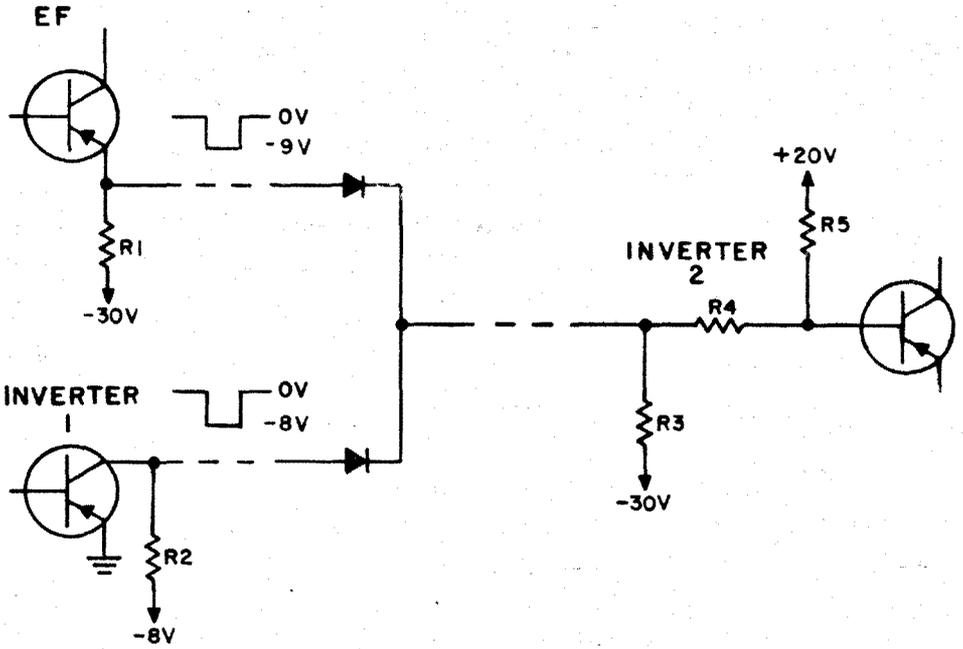
Figure 4-1. Typical "AND" Gate Connection
