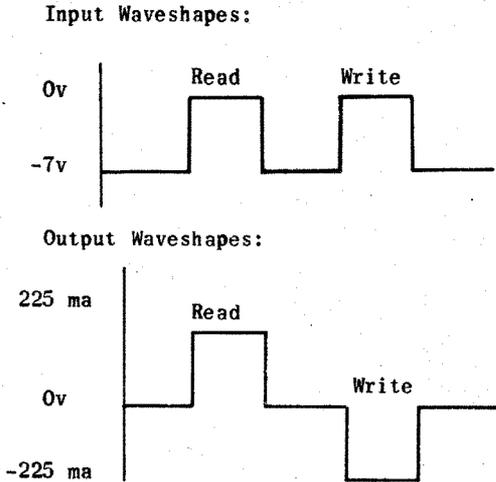
(1) CIRCUIT FUNCTION. - The current generator supplies the read and the write driving currents necessary to operate or switch the selected cores of the core stack. Each generator supplies both the X and the Y driving currents to one seven-plane core stack.
