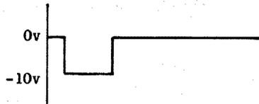
(1) CIRCUIT FUNCTION. - The delay line driver is triggered by the leading edge of the clock pulse (PTP2M) received from the processor. The driver generates a -10 volt, 800 nanosecond pulse which is applied to the 4 microsecond memory timing delay line.
