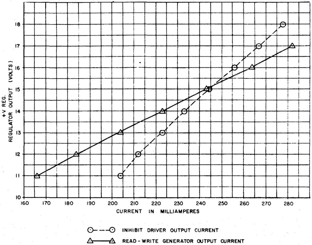
Figure 4-3b. Read/Write and Inhibit Current vs +V Reg
