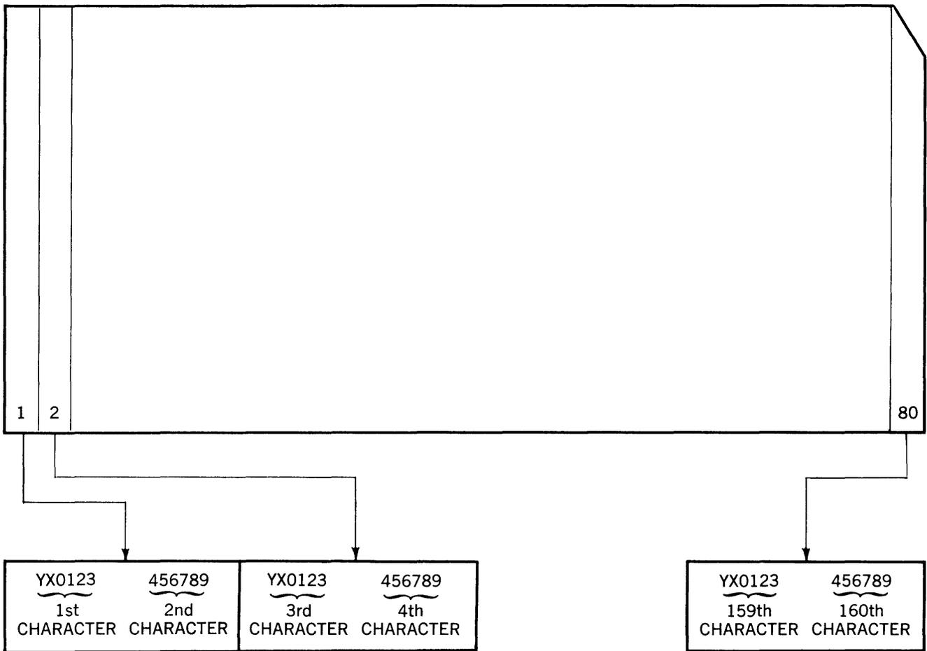
With a 90-column unit no translation is provided. The control unit can transmit data from a stub card. The number of characters of storage required for the 90-column card is 90.
