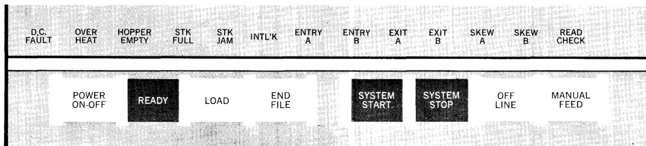
Figure 8-2. Card Punch Unit Control Panel.
