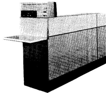
The Central Processor houses the control, arithmetic, storage, indexing, and other processing components which, operating at program direction, perform the input-output, logical and arithmetic functions of the system.
