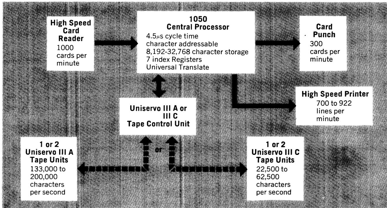
Figure 2-1. Block Diagram of a Typical System.
