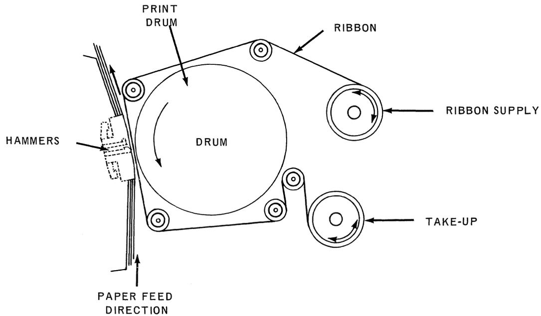
Figure A-4. Type 0751 Printer Mechanism
