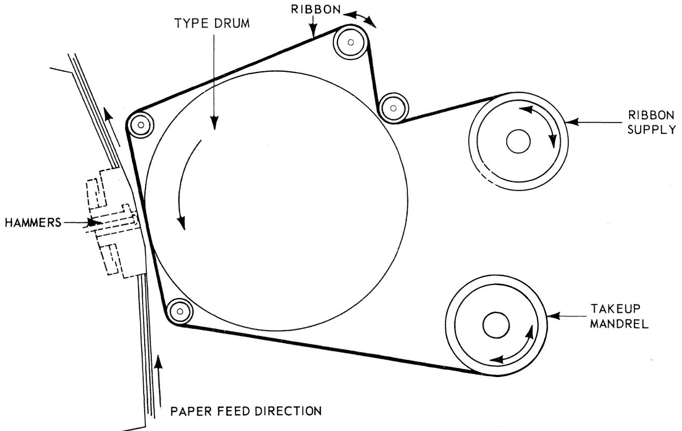
Figure 2-3. Printer Mechanism
