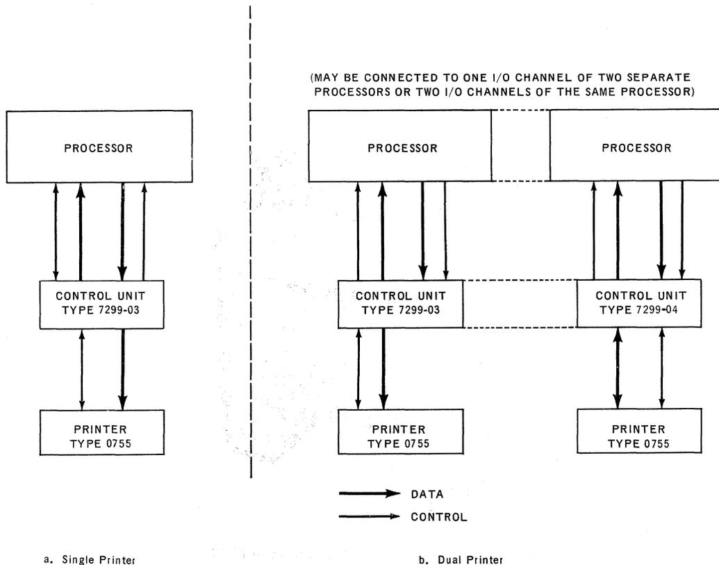
Figure 2-1. High Speed Printer Subsystem Configurations
