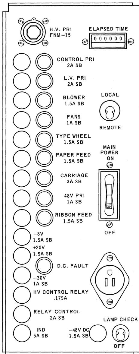
Figure A-3. Printer Power Control Panel
