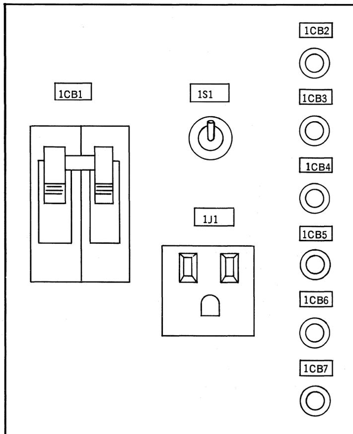
Figure 4-3. Printer Power Control Panel
