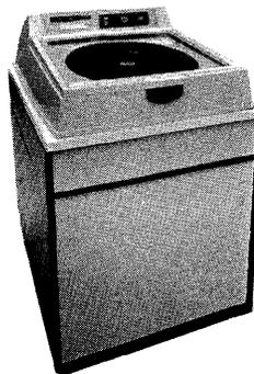
The UNIVAC 8414 Disc Subsystem offers a large storage capacity of up to 39.44 million 36-bit words of data online. A single disc pack provides for 5.0 million 36-bit words.
