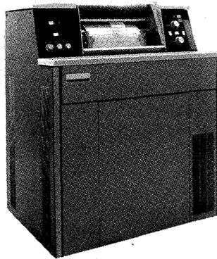
The UNIVAC multiple high-speed printer subsystem provides the UNIVAC 1110 System with an output printing unit that is capable of printing single or multiple copies of data. Each line of output data may contain up to 132 printed characters. Printing operations which occur on a request/acknowledge basis allow the processor to perform other processing functions while the printer is printing data.
