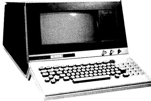
The UNISCOPE 100 Visual Communication Terminal Subsystem is a low-cost, alphanumeric display designed for a broad range of applications which require direct operator interaction with a centralized computer system. Due to its modular construction, the UNISCOPE 100 terminal can operate either as a data entry or as a display device. It can be conveniently located at the central computer site or at a remote station where it is connected to the system by way of telephone lines.
