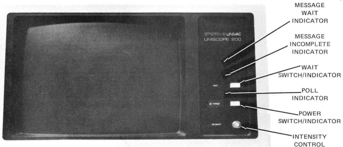
b. UNISCOPE 200 Display Terminal, Front View
