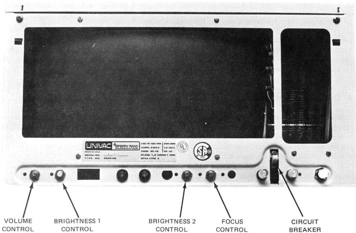
Figure 3-5. UNISCOPE 100 Display Terminal, Front View with Faceplate Removed
