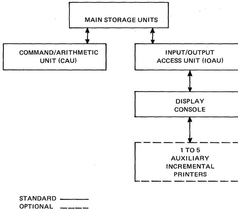
Figure 2-1. UNIVAC 1110 and SPERRY UNIVAC 1100/40 Systems, Central Group Unit Processing Configuration
