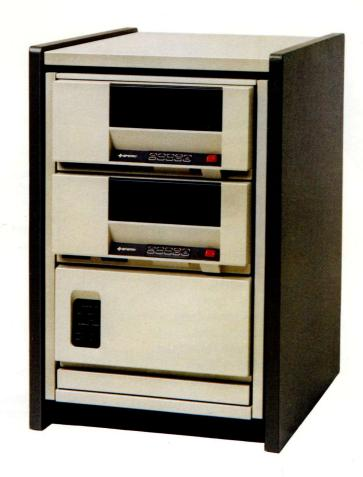
The SPERRY F3782 Streaming Magnetic Tape Unit is a new concept in magnetic tape devices for Sperry. The technology utilizes half inch magnetic tape moving between tape reels without the use of vacuum columns. The design of the tape transport contributes to a low cost, high speed device that is a cost effective alternative as a dump/restore device for fixed media disk drives.
