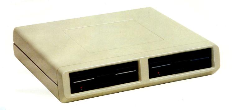
The SPERRY 8439 double-sided diskette subsystem is a freestanding peripheral device that provides random access mass storage using inexpensive 51/4-inch diskettes. The low-profile diskette drives are packaged in an attractive and functional enclosure, suitable for desk-top operation.
