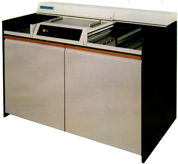
The newest SPERRY UNIVAC® 0716 (80/96-column) card reader subsystem offers reliability, versatility, easy operation and low cost. 80-column cards or 96-column cards are read at rates of 600 or 1000 per minute. 66- and 51-column card operation is available.
