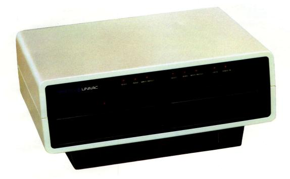
The SPERRY UNIVAC 8406 double-sided diskette subsystem is a freestanding peripheral vice which provides random access mass storage, packaged for desk-top operation. It utilizes an inexpensive, easy-to-use reuseable flexible diskette as the storage medium and provides a storage capacity of up to 1 M bytes per diskette. Up to 2 drives can be configured per subsystem.
