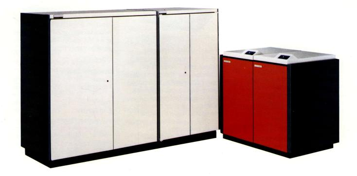
The SPERRY UNIVAC® Cache/ Disk System (C/DS) is an I/O hierarchical mass storage system incorporating a technology and architectural concept that provides a system offering significant I/O performance advantages for the SPERRY UNIVAC 1100/80 and 1100/60 Systems. The use of semiconductor storage in conjunction with large capacity fixed disk storage will permit frequently used data to be automatically stored in solid state memory to provide "data acceleration" via the improved access time.
