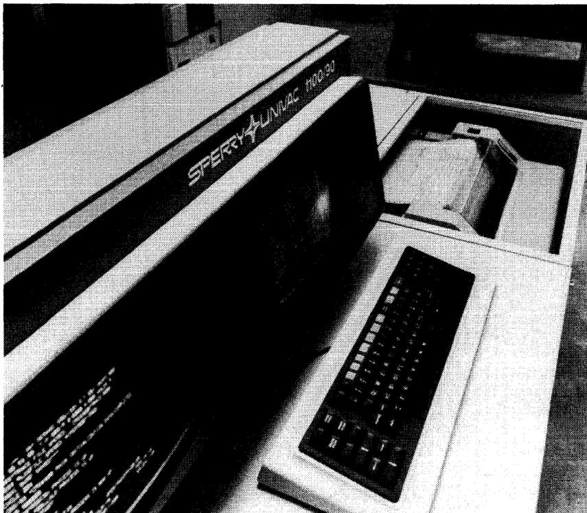
*The most recent addition to the 1100 Series of large-scale systems is the 1100/90 System. With double the main memory capacity of the 1100/60 and 1100/80, the 1100/90 provides a new virtual machine capability, and features a number of extensions to the 1100 Series architecture.*
